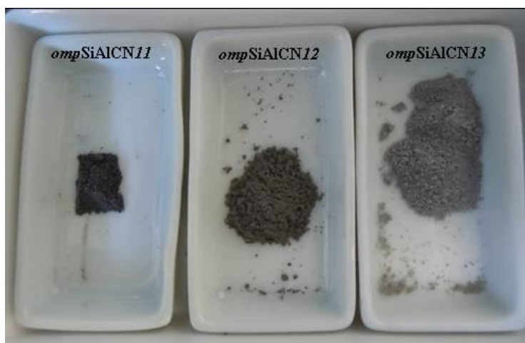
Figure IV-11 : ompSiAlCN xy samples after template removal.
