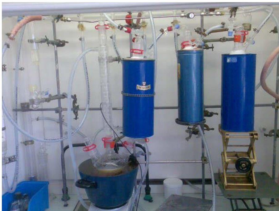
Figure III-1: Experimental procedure for borazine synthesis.
