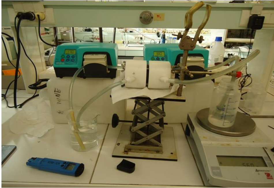
Figure 112. Custom made forward osmosis filtration system
