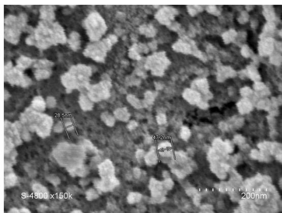
**Figure 95.** SEM image of a dried **HC8** nanocrystal solution containing particles in the range 30-70 nm
