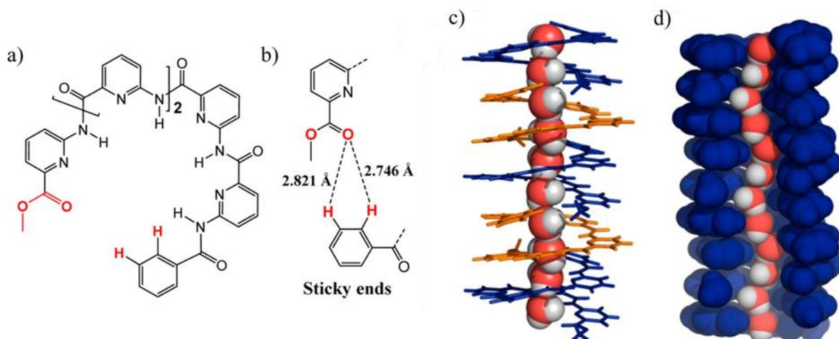
**Figure 10.** a) Building block of the synthetic water channels; b) “sticky ends” motif for self-assembly guidance; c) crystal structure and d) representation of a single water channel (image adapted from reference [53])
