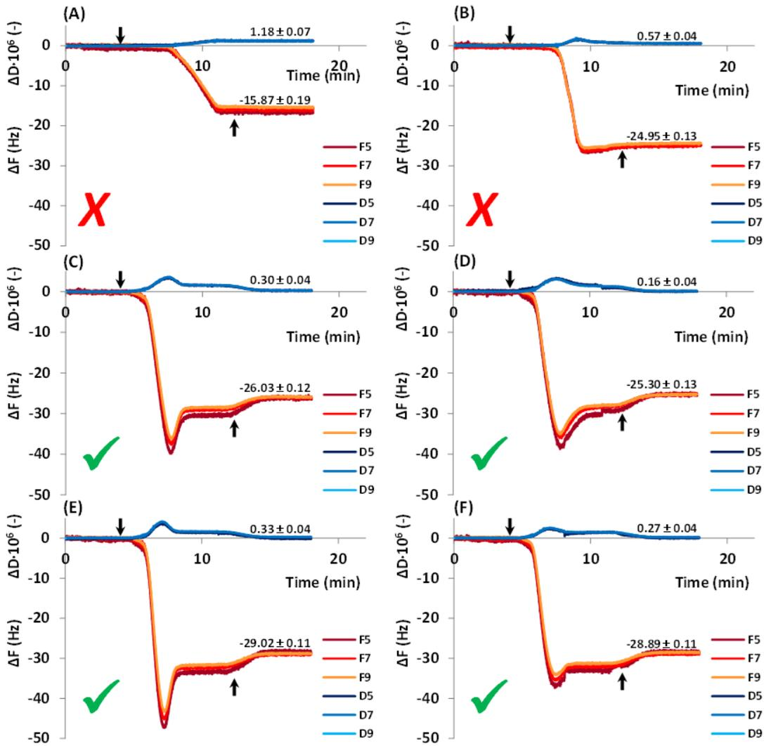
**Figure 45.** Lipid vesicles deposition for (A) POPC, (B) POPC + **HC8**, (C) 4:1=POPC:DOPS, (D) 4:1=POPC:DOPS + **HC8**, (E) 4:1=POPC:DOPS, 20% w/w Chol and (F) 4:1=POPC:DOPS, 20% w/w Chol + **HC8**. The two arrows indicate (i) lipid vesicles injection and (ii) washing step with 10 mM phosphate buffer pH 6.4
