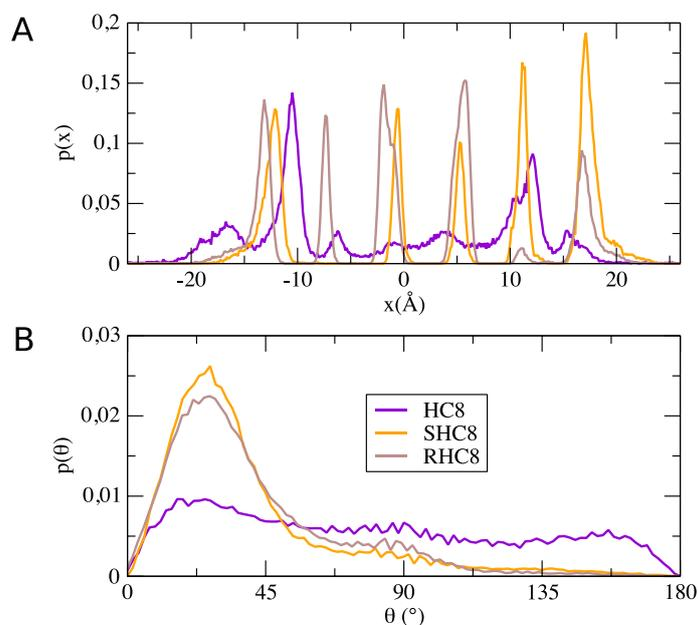
**Figure 48.** A. One-dimensional water density profile for crossing water averaged for the simulations of the **HC8**, **R-HC8** and **S-HC8** channels at 10 atm. B. Water dipolar moment orientation with respect to the z-axis perpendicular to the membrane – only channel water is used for this calculation.
