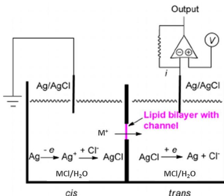
**Figure 64.** Schematic of a bilayer patch clamp setup
