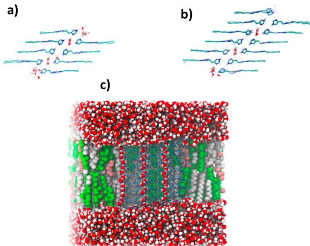
**Figure 31.** Schematic top and side views of the a) WC4 system and the b) larger 12x8 WC6 system used as starting point for all simulations; c) membrane packing and water filling in the simulation box
