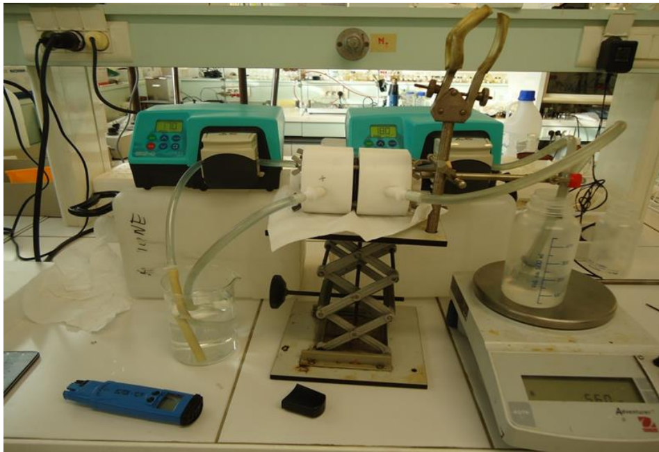
Figure 112. Custom made forward osmosis filtration system
