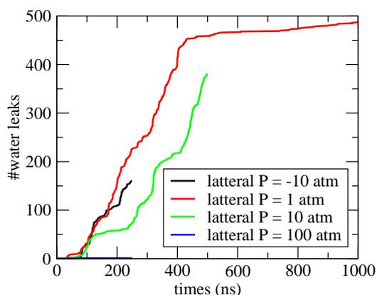
**Figure 46.** The water transport activity time series of the **HC6** channels under increasing lateral pressure, from -10 atm to 100 atm is shown. Cumulated transport of water molecules across the membrane, in either direction, is shown.
