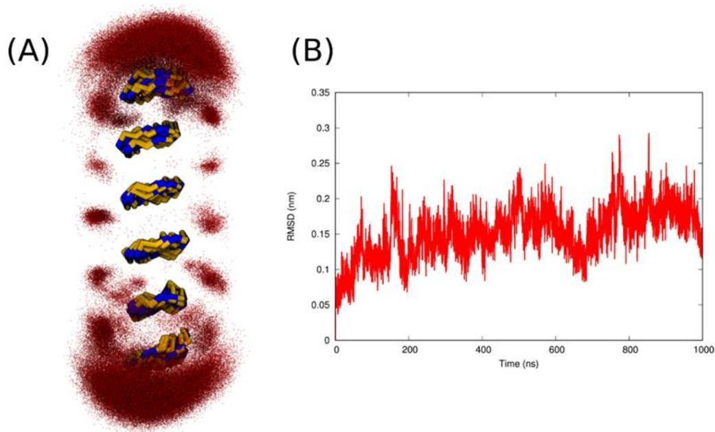
**Figure 70.** (A) - Water density around the DOTA central ring stack. Water oxygen atoms were represented as red dots overlaid for multiple frames during simulation. (B) – RMSD of DOTA stack with respect to the starting configuration.
