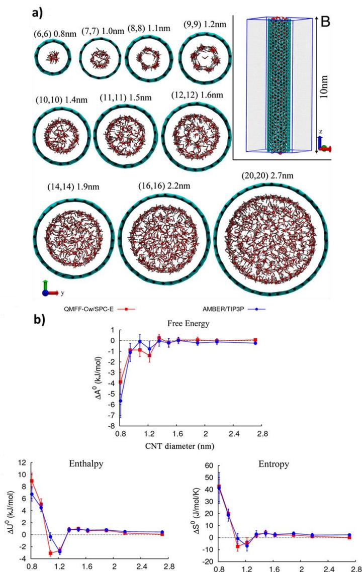
**Figure 8.** a) Water structuration in a 10 nm long CNT with varying pore sizes obtained through equilibrium molecular dynamics b) variation of free energy, enthalpy and entropy of water confined in CNT pores of varying size using two different simulation models (image adapted from reference [33])
