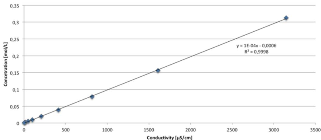
**Figure 111.** Calibration curve of Hanna conductivity meter
