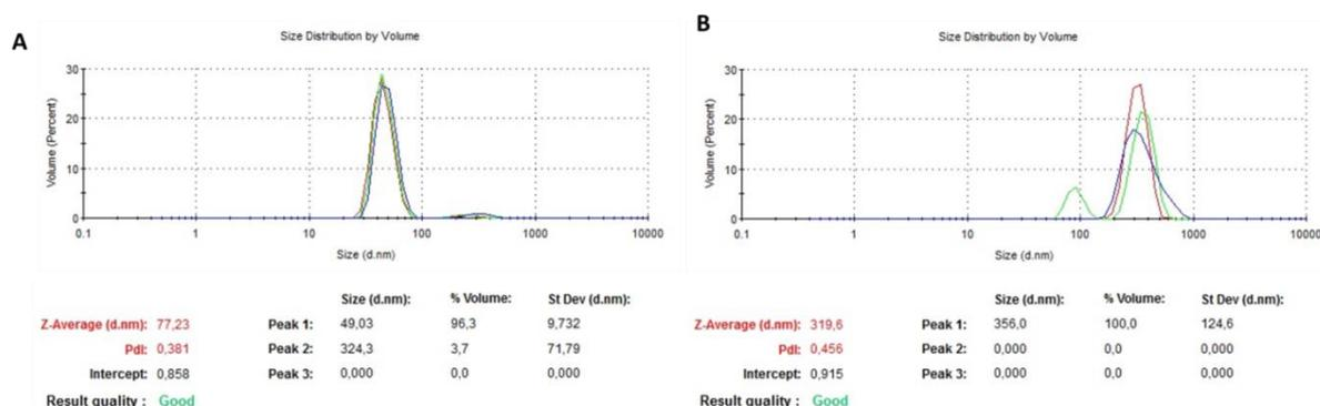
**Figure 108.** Dynamic light scattering results for (A) 1 mM nanocrystal solution and (B) 2 mM nanocrystal solution
