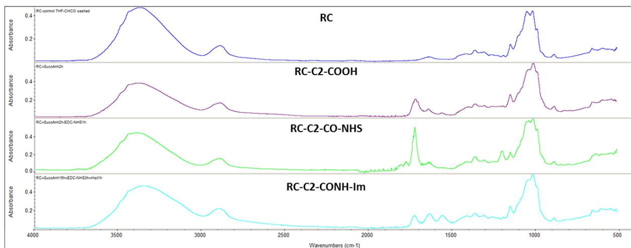
**Figure 105.** ATR-FTIR spectra of step-by-step functionalization of RC membranes
