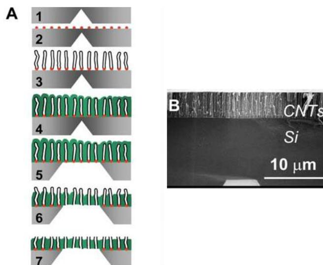
**Figure 9.** (A) CNT membrane fabrication: 1) silicon support micro etching 2) catalyst deposition 3) nanotube growth 4) gap filling with chemical vapor deposition 5) membrane area etching 6) ion etching to expose nanotubes and remove catalyst nanoparticles 7) nanotube uncapping (B) SEM cross-section of the CNT membrane (Image adapted from reference [30])
