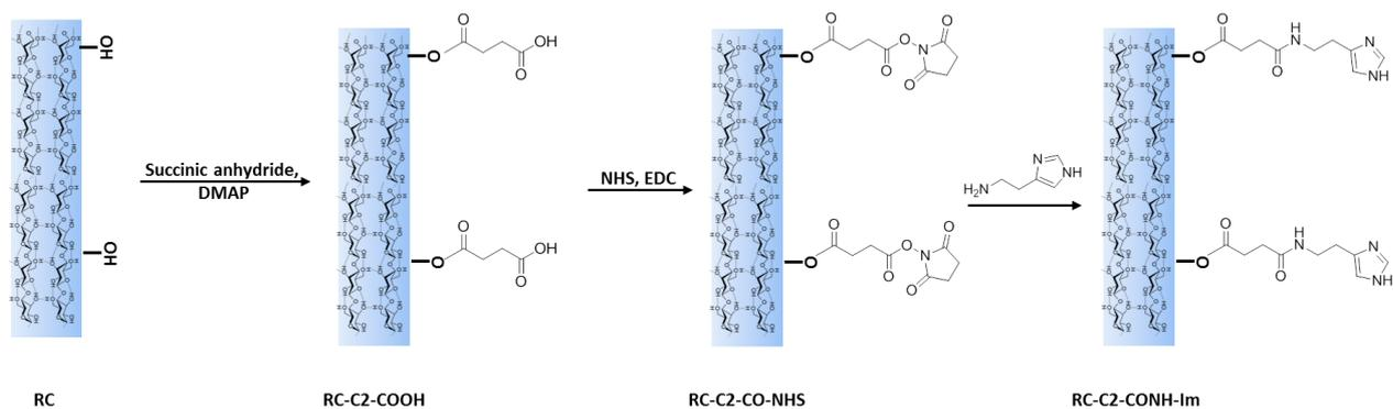
**Figure 104.** Step-by-step grafting of RC membranes
