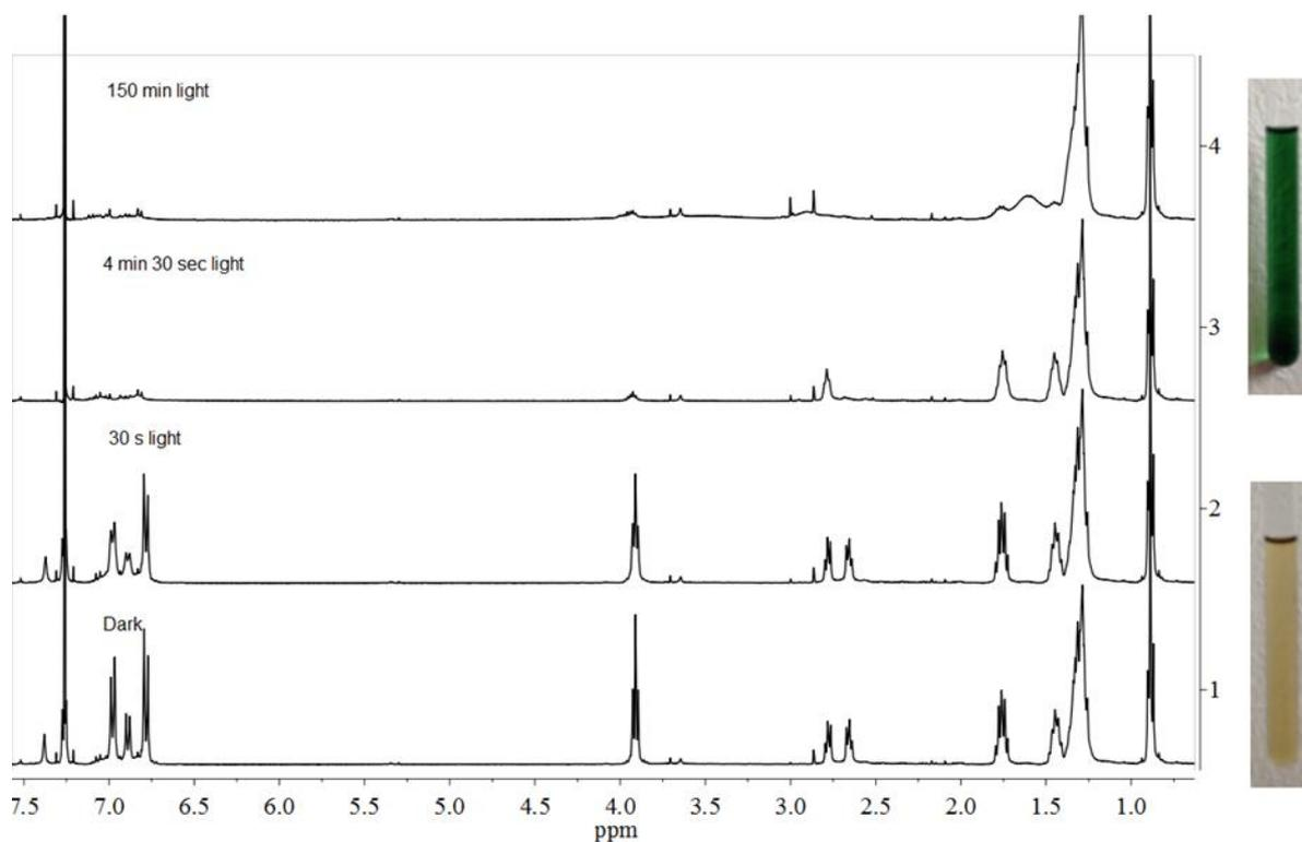
**Figure 75.** Change in <sup>1</sup>H-NMR during light irradiation of a 1mM CDCl<sub>3</sub> solution of compound **TAA1**.
