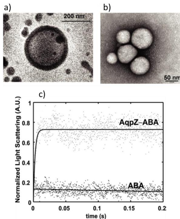
**Figure 4.** Cryogenic transmission electron micrograph of a polymer vesicle b) electron micrograph of a cluster of vesicles c) Stopped-flow light-scattering experiments; increase in relative light scattering with and without reconstituted AqpZ into the polymer at 5.5°C at a molar ratio of 200:1 (polymer:protein) (image adapted from reference[21])
