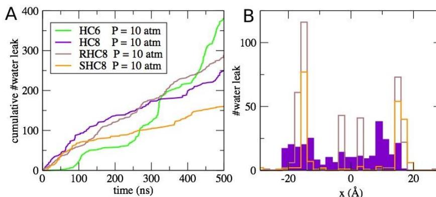
**Figure 36.** (A) The water transport activity time series of the I-quartet channels is shown as the cumulated passage of water molecules across the membrane, in either direction (B) shows the count of permeation events for each water wire along the membrane width (x-axis).
