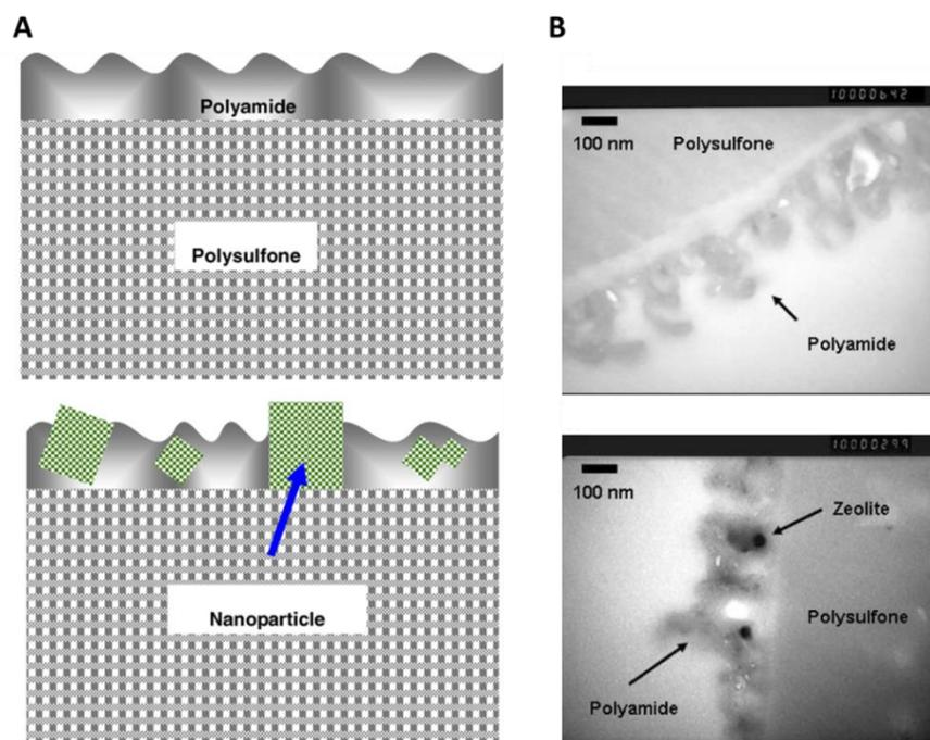
**Figure 93.** (A) Polyamide TFC and TFN with zeolite nanoparticles and (B) TEM images of the membranes (image adapted from reference [113])
