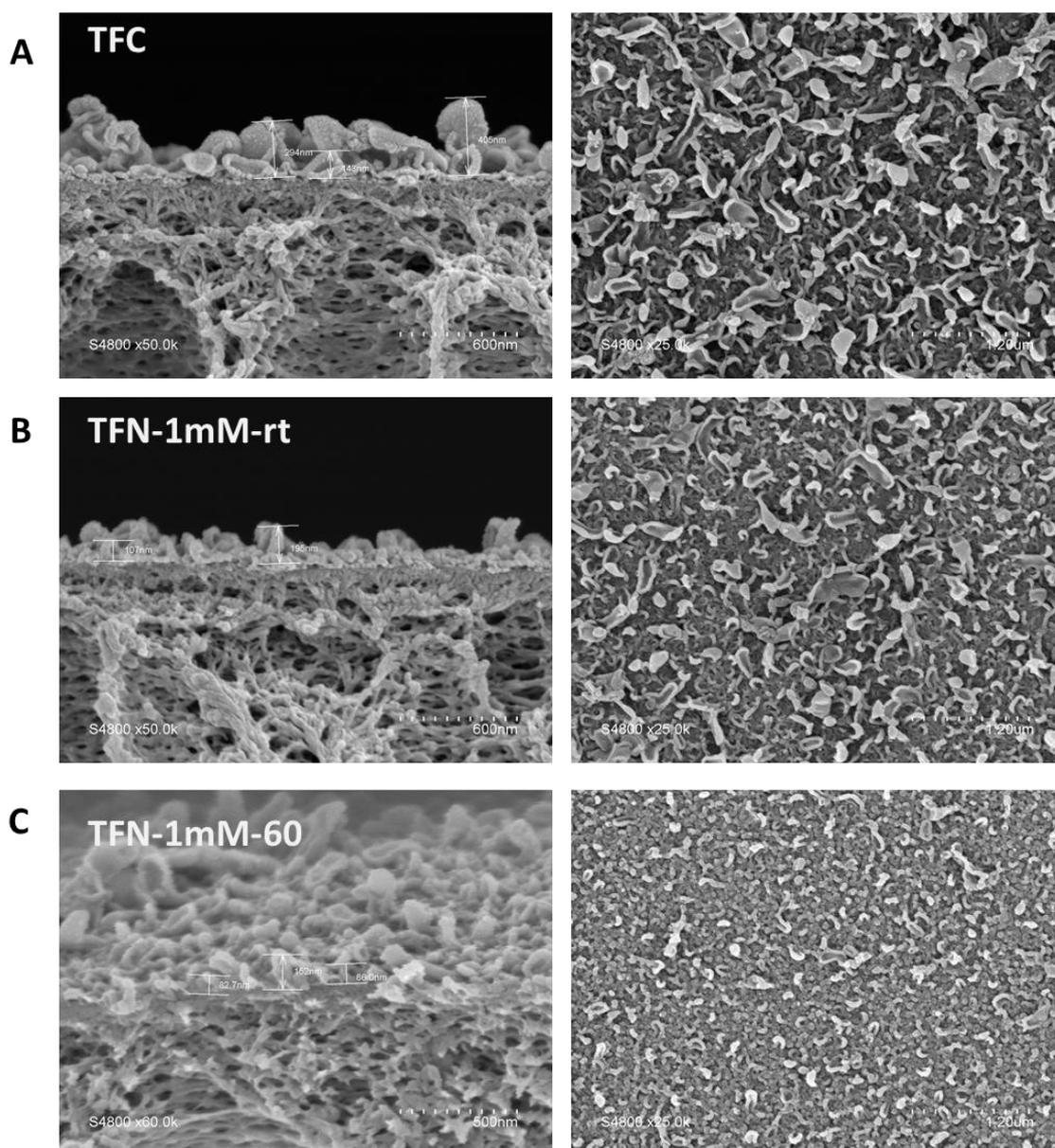
**Figure 96.** Cross-section and surface SEM images of (A) TFC control membrane, (B) TFN with nanocrystal solution obtained at room temperature and (C) TFN with nanocrystal solution obtained by recrystallizing from 60°C HC8 solution
