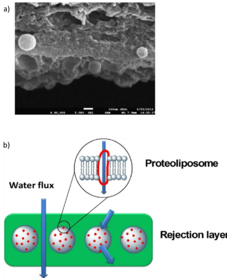
**Figure 5.** a) Scanning electron microscopy (SEM) image of the cross-section of an ABM-thin film composite membrane b) Conceptual model of aquaporin proteoliposomes integrated into a polyamide rejection matrix (image adapted from reference[23])
