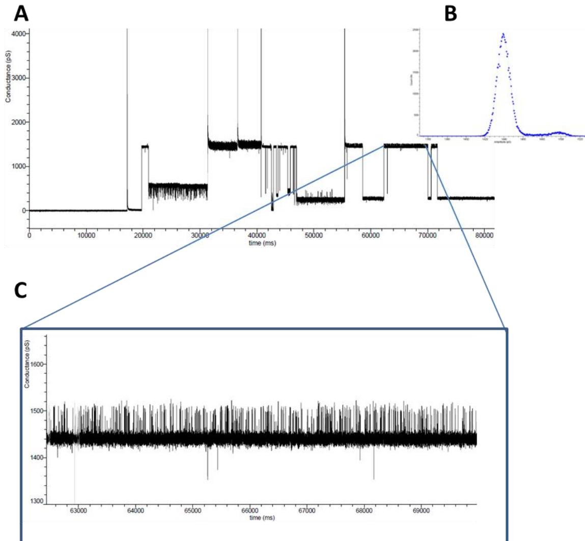
**Figure 65.** Registered conductance variation across flat sheet lipid bilayer under addition of Dota6. (A) Multimodal behavior; (B) conductance histogram and narrow Gaussian fit; (C) Flickering activity between two open states
