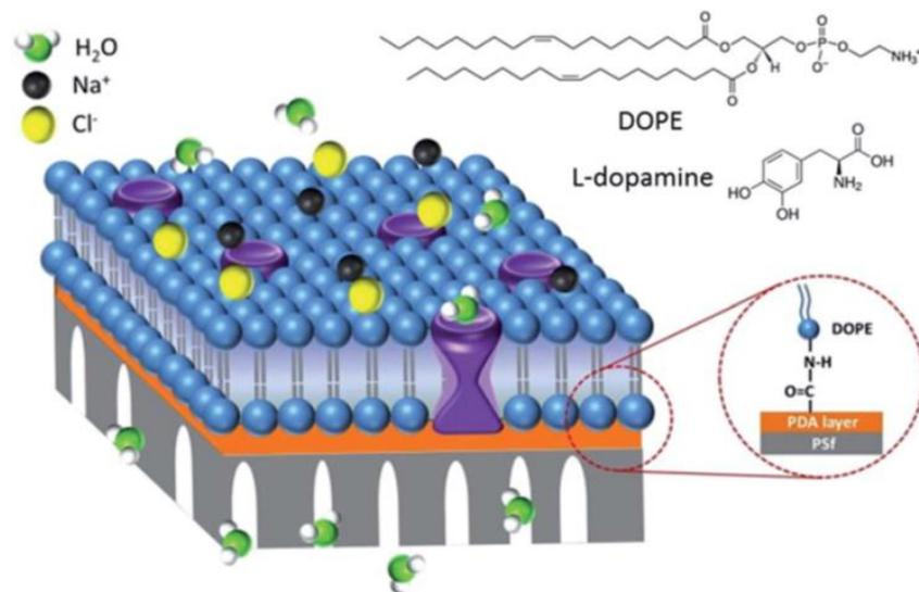
**Figure 3.** Schematic presentation of the structure of the AqpZ-incorporated SLB membrane with covalent bonds; the amide bond linked 1,2-Dioleoyl-*sn*-glycero-3-phosphoethanolamine (DOPE) SLB is established on top of a polydopamine (PDA) layer (orange) coated porous polyethersulfone (PSf) (gray) support (image adapted from reference [20])
