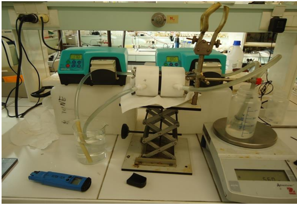
Figure 112. Custom made forward osmosis filtration system
