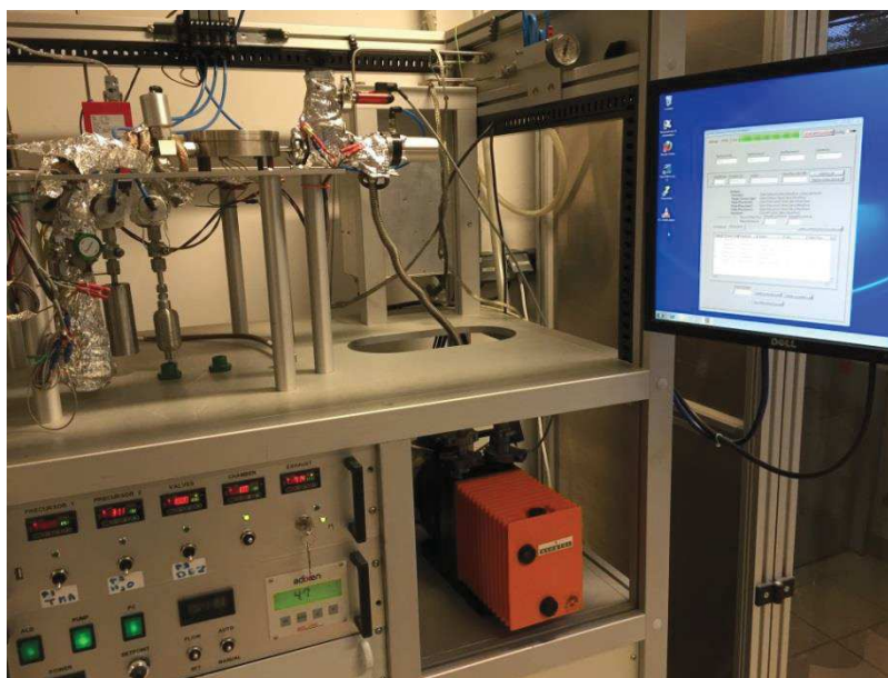
Figure 2-23. Atomic layer deposition reactor.
