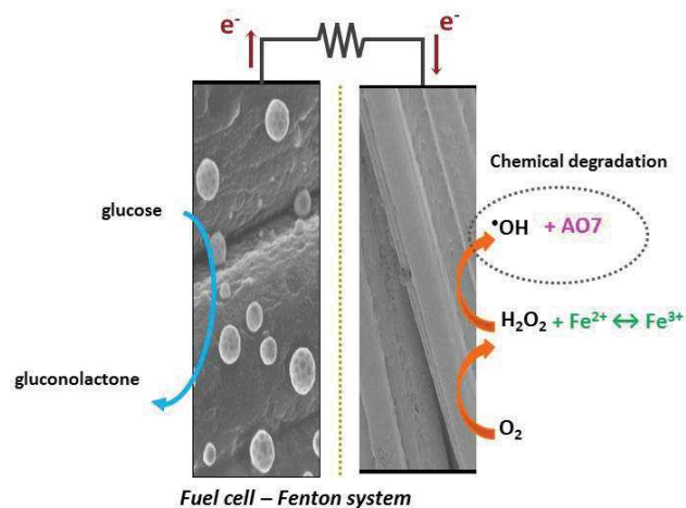
Figure 6-1. Schematic diagram of the FC-Fenton based system.
