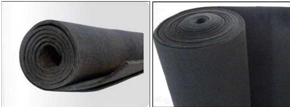
Figure 2-1. Typical shape of commercial (a) CF and (b) GF [31].
