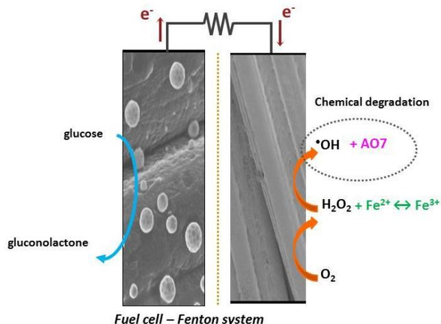
Figure 6-1. Schematic diagram of the FC-Fenton based system.
