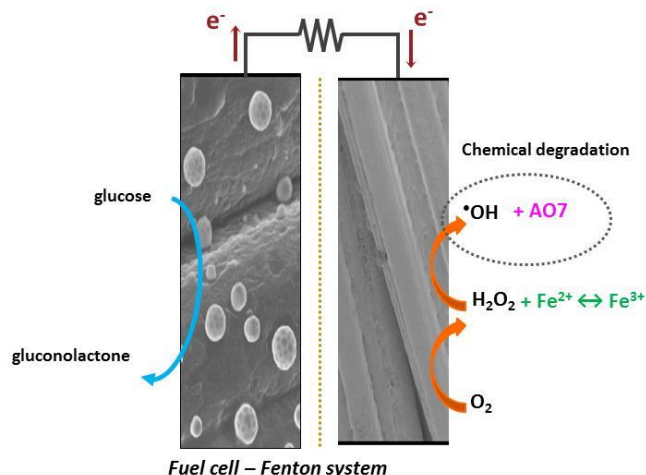
Figure 6-1. Schematic diagram of the FC-Fenton based system.
