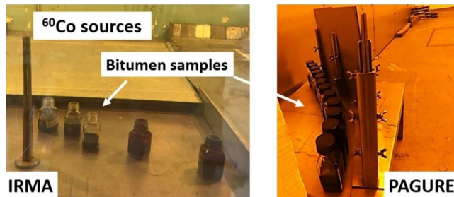
Fig. 1. Bitumen samples irradiated in IRMA and PAGURE facilities.
