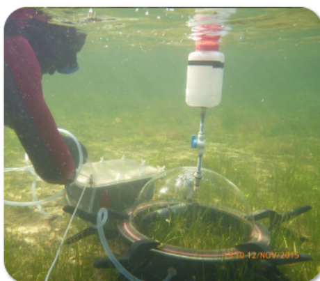
Figure. 3 - Benthic chamber in use during light incubation. The same model with a dark dome was used to measure respiration. ©IFREMER
