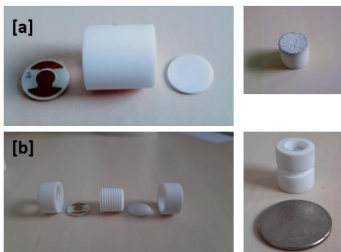
Figure 4 : [a] Design n°1 before and after the sealing step with alumina cement [b] Design n°2 of the screwed version before and after its assembly
