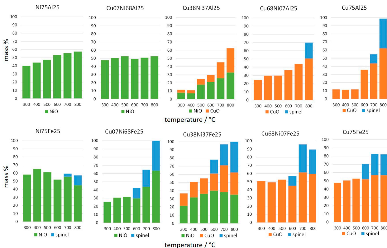
Figure 10. Mass % of phases in samples of the series (Cu,Ni)Al ( top ) and (Cu,Ni)Fe ( bottom ) as a function of temperature in XRD thermal ramp: NiO bunsenite (green), CuO tenorite (red), and spinel (blue).
