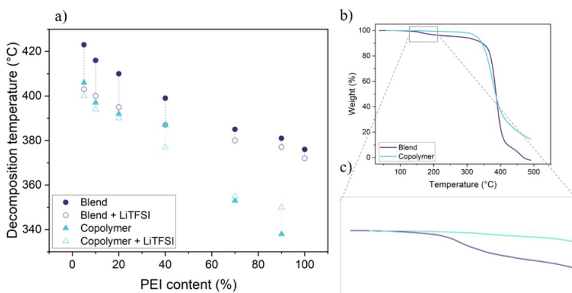
**Figure 4.** a) Decomposition temperature for PO<sub>x</sub>:BPEI blends and PO<sub>x-co</sub>-PEI copolymers versus PEI content with or without Li salt by using ATG technic, b) ATG curve of PO<sub>x60</sub>:BPEI<sub>40</sub> and PO<sub>x60-co</sub>-PEI<sub>40</sub> with a c) zoom on the region of 100-200 °C.
