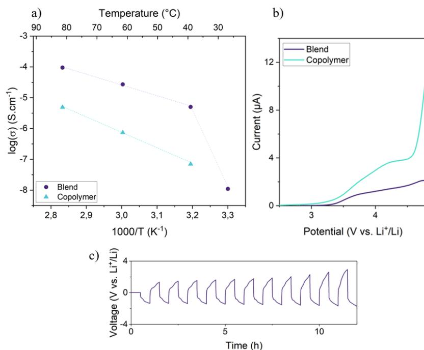
**Figure 6.** a) Conductivity related to the temperature of  $\text{POx}_{10}:\text{BPEI}_{90}$  and  $\text{POx}_{60}\text{-co-PEI}_{40}$ , b) Stability window in potential of  $\text{POx}_{10}:\text{BPEI}_{90}$  and  $\text{POx}_{60}\text{-co-PEI}_{40}$  and c) voltage in function of time for  $\text{POx}_{10}:\text{BPEI}_{90}$  in lithium symmetric cell.
