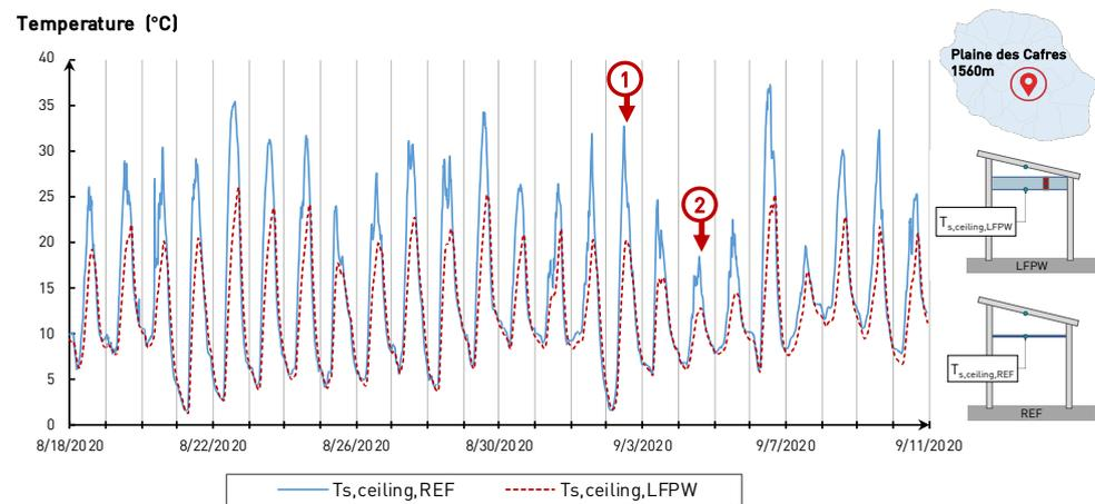
**Figure 9.** Evolution of the surface temperature of the ceiling during the first part of the measurement period.
