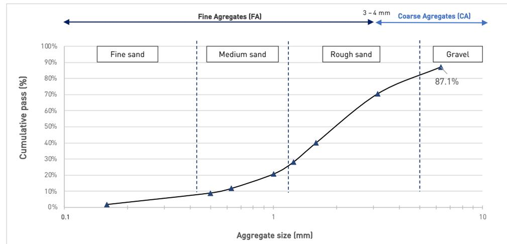
**Figure 6.** Size analysis of the loose-fill plastic waste with aggregate size equivalence.
