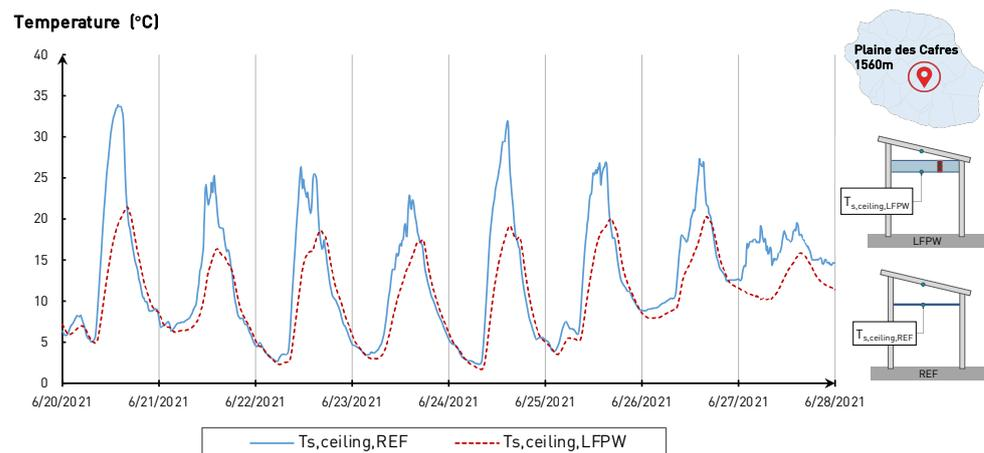
**Figure 10.** Evolution of the surface temperature of the ceiling during the coldest week of the second part of the measurement period.
