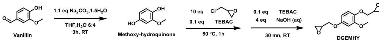
Figure 7 - Reaction scheme for the synthesis of DGEMHY starting from vanillin according to Fache et al. 41
