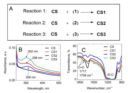
Fig. 2 A Scheme of synthesis of CS nanoparticles grafted with *trans*-resveratrol. B UV–Vis spectra of the 3 types of grafted nanoparticles from 240 to 510 nm. C The infrared spectra of core/shell grafted with 1, 2, 3 molecules corresponding to CS1, CS2, and CS3, respectively. Both UV–Vis and IR spectra of native CS (black curves) were plotted to observe the changes in absorbance and transmittance properties of the nanoparticles
