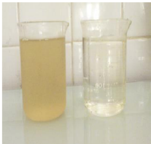
Figure 10: showing the color of the effluent before (A) and after treatment (B).
