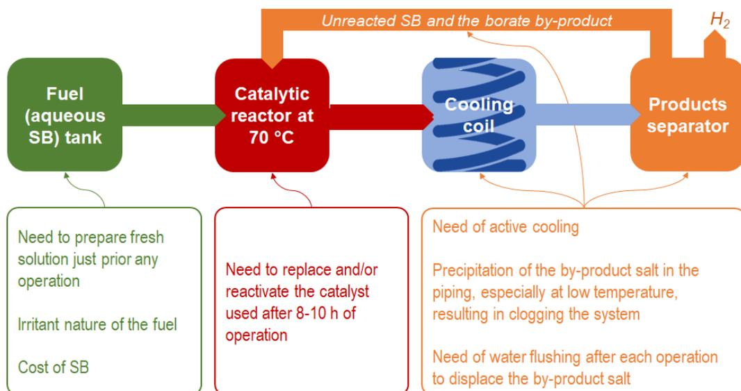
**Figure 6.** The recurring issues encountered by a H<sub>2</sub> production system, as reported by Lapena-Rey et al. [100].
