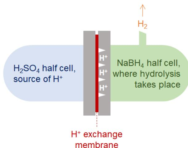
**Figure 4.** Scheme of the H<sub>2</sub> production system, based on two half-cells, as proposed in ref. [87]. The H<sub>2</sub>SO<sub>4</sub> half cell is separated from the SB half cell by a proton exchange membrane (disulfonated poly(arylene ether sulfone) copolymer), and the H<sub>2</sub> produced in the latter cell is vented through an outlet.
