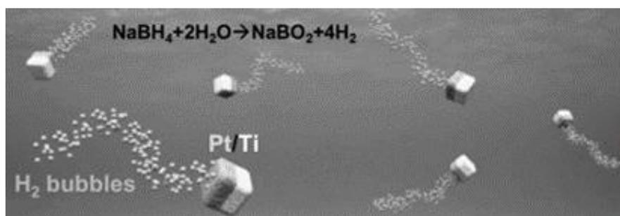
**Figure 3.** Schematic representation of the Pt-black/Ti Janus micromotors by the production of H<sub>2</sub> microbubbles by hydrolysis of SB. Reproduced from ref. [74] with permission granted by John Wiley and Sons (January 6, 2023).
