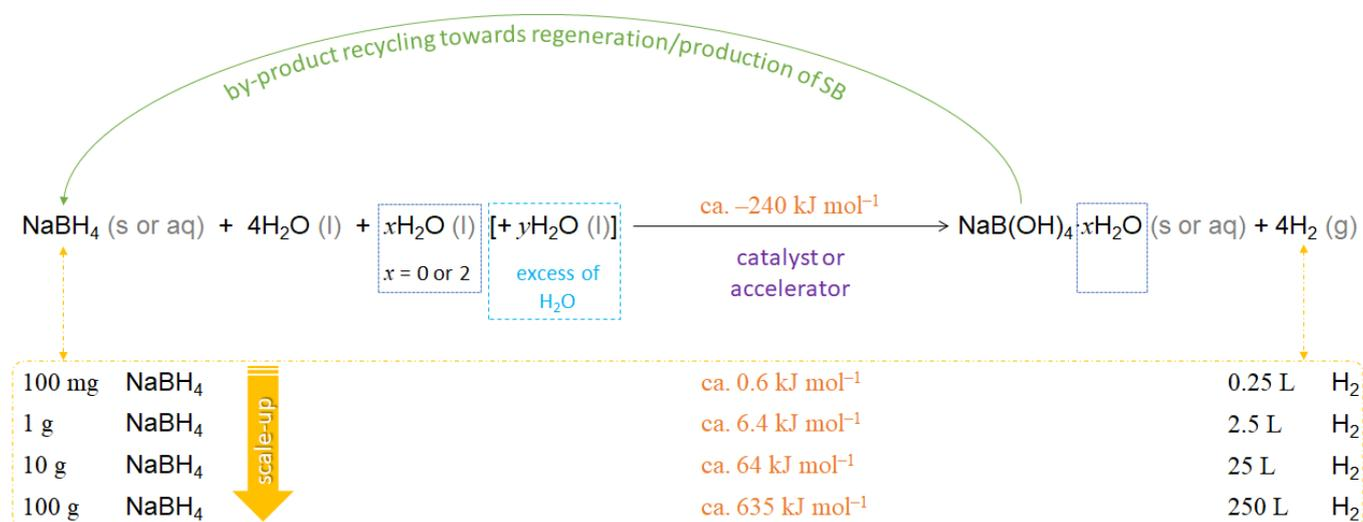
**Figure 1.** Hydrolysis of SB: the reactants, water in excess as solvent, a catalyst or an accelerator, the heat of the reaction, the by-products, the product H<sub>2</sub>, and the amounts of SB and H<sub>2</sub> towards scale-up.
