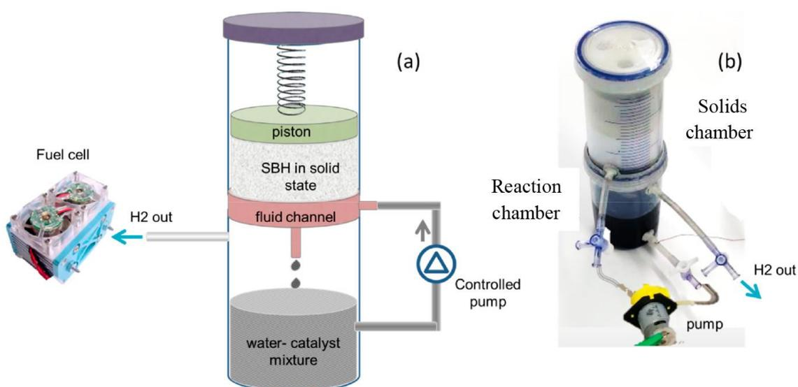
**Figure 5.** Avrahami and co-workers' pump-based circulation generator: (a) schematic concept (with SBH for sodium borohydride as denoted by the authors); (b) photograph of the generator described in (a). Reprinted with permission from reference [106]. Copyright 2021 American Chemical Society.
