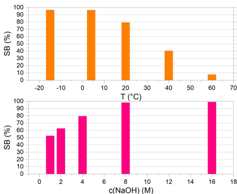
**Figure 2.** SB remaining (in mole percentage) in aqueous alkaline solution after a storage of 12 weeks: (top) effect of the temperature ( $-15$ ,  $4$ ,  $20$ ,  $40$  and  $60$  °C) for an aqueous solution of SB (initial concentration of  $4$  M) having a concentration of NaOH of  $4$  M; (bottom) effect of the initial concentration of NaOH ( $1$ ,  $2$ ,  $4$ ,  $8$  and  $16$  M) for an aqueous solution of SB (initial concentration of  $4$  M) stored at  $20$  °C.
