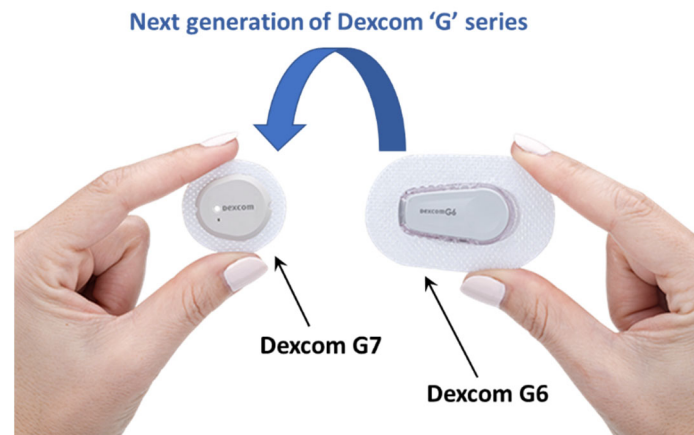
Figure 6. Size evolutionary of Dexcom G6 to G7 wearable transmitter (adapted from Dexcom website: https://www.dexcom.com/ ).
