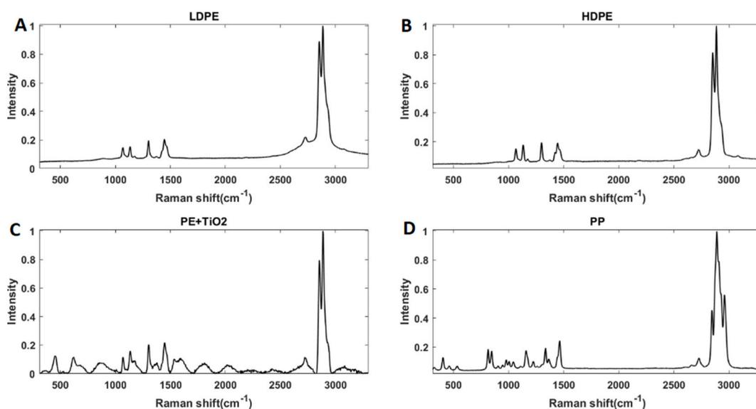
**Fig. 2.** Micro-Raman spectra of the four types of polymers (A: LDPE/Low Density Polyethylene; B: HDPE/High Density Polyethylene; C: PE = TiO<sub>2</sub>/Polyethylene incrustated by TiO<sub>2</sub>; D: PP/Polypropylene) identified in the 27 samples collected in three different seasons in the three lagoons (Biguglia, Diana and Prevost). Sample identification was performed by comparing acquired spectra to reference spectra (see Materials and Methods).
