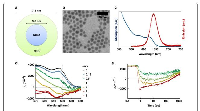
Fig. 1 Properties of the synthesized QDs. a Schematic structure of a core/shell CdSe/CdS QD. b TEM image. c Absorption spectrum (blue) and photoluminescence spectrum (red) of the QDs dispersed in toluene. d QD absorption ( $\mu_i > 0$ ) or gain ( $\mu_i < 0$ ) spectrum as a function of the excitation level < N > at 3 ps after the pulse excitation. e Corresponding time-dependency of the gain spectrum at a fixed probe wavelength of 630 nm
