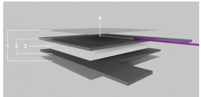
**Figure 1.** Placement of the microsphere-based fiber-optic sensor embedded in the supercapacitor in schematic cross-section where: 1 – covers, 2 - electrodes, 3 – separator, 4 – microsphere-based fiber-optic sensor.
