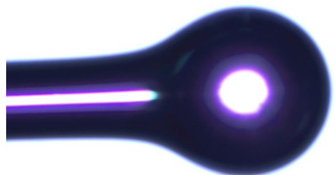
Figure 2. A microscope image of the microstructure used for supercapacitor in situ temperature measurement.
