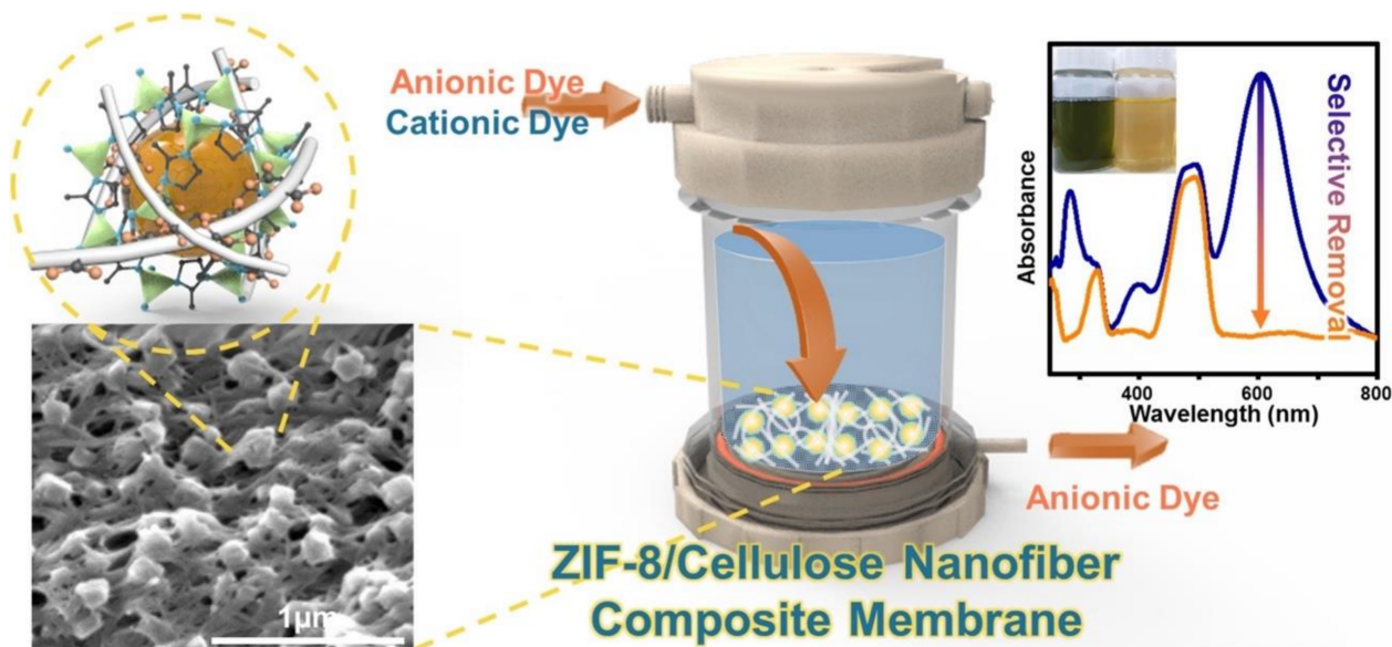
Figure 12. Control of the cellulose nanofibrous composite membrane structure by in-situ synthesis of zeolitic imidazolate framework-8 (ZIF-8) at cellulose nanofibers (CNF) for the selective removal of cationic dyes [235], © Elsevier, 2019.
