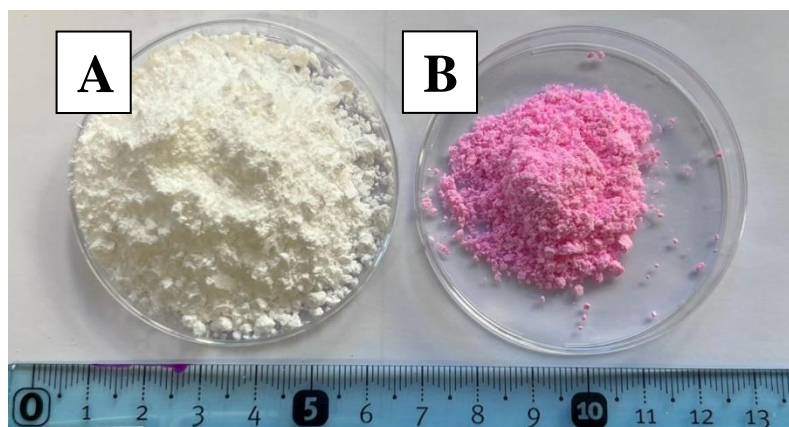
Figure 2. (A) dried PCL/DMF microspheres in the form of a powder without any addition, (B) dried rhodamine-loaded PES/NMP microsphere powder.
