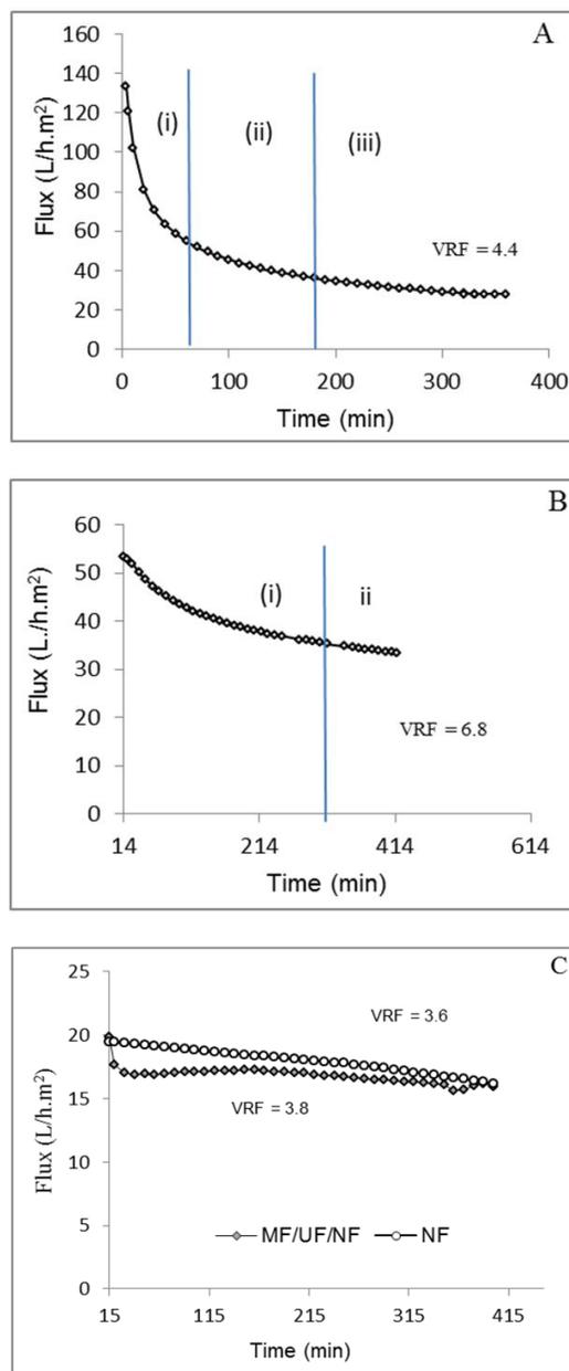
**Fig. 6. Schematic representation of kola extract filtration at 25°C (A) microfiltration, TMP =1 bar, CFV=2 m/s, flow = 150 l/h), (B) ultrafiltration, TMP =3 bar, CFV= 2 m/s, flow = 150 l/h), (C and D) nanofiltration, TMP =10 bar, FV=1 m/s, flow =120 l/h)**
