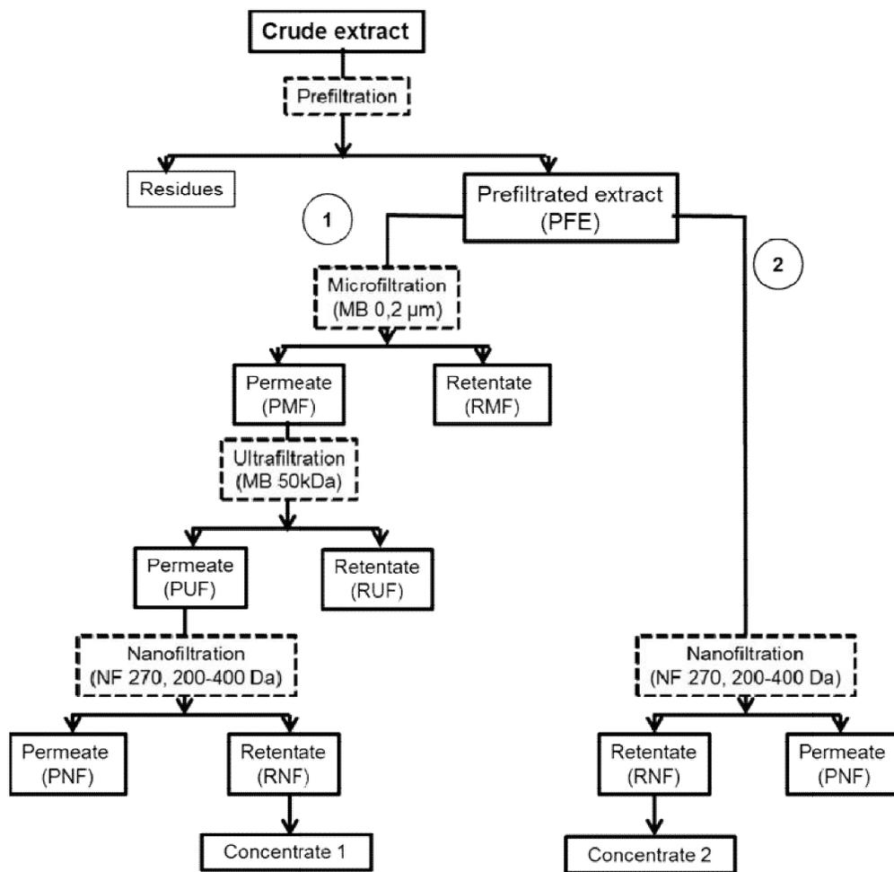
Fig. 2. Preparation of concentrated kola extracts: Schematic flow sheets of the membrane processes
