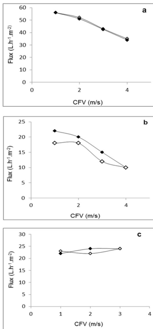
**Fig. 4. Effect of initial permeate flux on molecules fouling for various crossflow velocities: (◆) low to high crossflow and (◇) high to low crossflow. Results are presented flux vs cross-flow: (a) microfiltration, TPM = 1 bar, T = 25°C, Q = 150 l/h, (b) ultrafiltration, TPM = 2 bar, T = 25°C, Q = 150 l/h (c) nanofiltration, TPM = 10 bar, T = 25°C, Q = 120 l/h**
