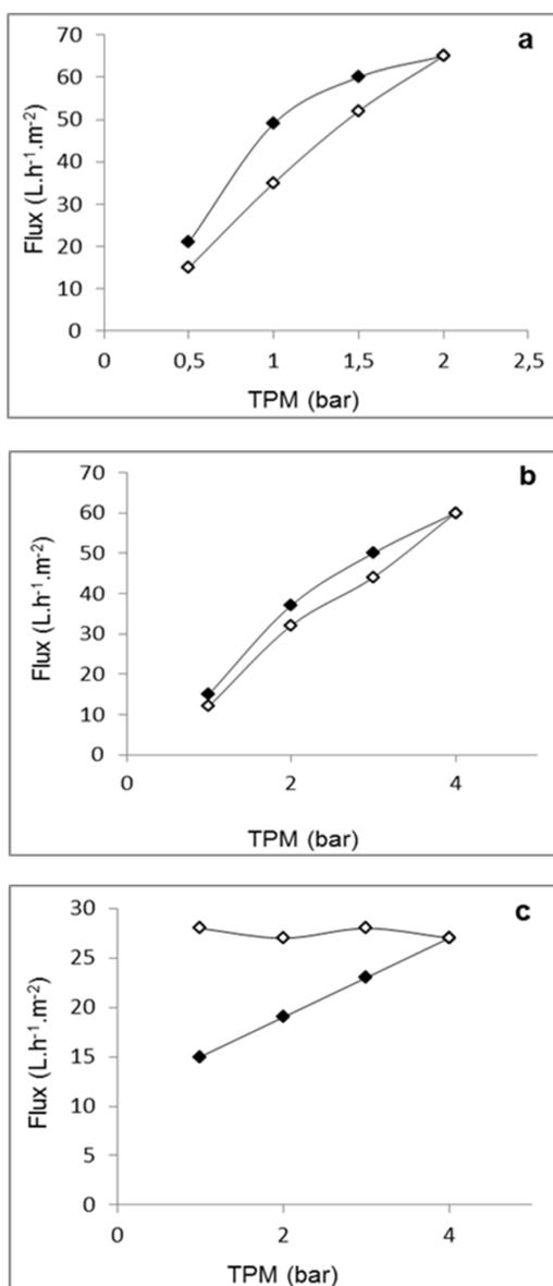
**Fig. 5. Effect of initial permeate flux on molecules fouling for various pressures: (◆) low to high pressure and (◇) high to low pressure. Results are presented flux vs pressure: (a) microfiltration at 2 m/s, (b) ultrafiltration at 2 m/s, (c) nanofiltration at 1 m/s**
