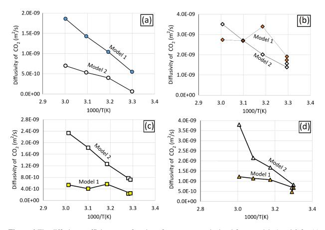
**Figure 4** The diffusion coefficients as a function of temperature calculated from models 1 and 2 for (a) [emim][Ac], (b) [emim][DCA], (c) [emim][MeSO<sub>4</sub>], and (d) [emim][EtSO<sub>4</sub>]. The colored data represent the predictions by model 1 (transient thin-film), and the open data show the predictions of model 2 (semi-infinite volume).
