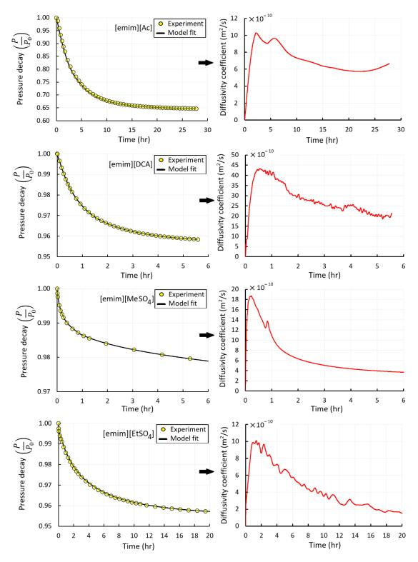
**Figure 5** Adjusted diffusivity coefficients for the experiments of the diffusion of CO<sub>2</sub> in four ILs at 313.15 K. The diffusivity coefficient in eq. 16 is adjusted so that the predicted pressures in the gas phase (left plots) match the measured ones.
