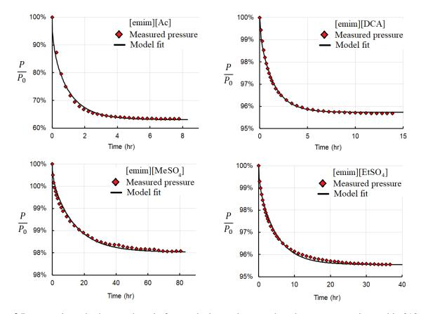
Figure 3 Pressure decay in the gas phase in four typical experiments when the temperature is roughly 313K (From Table 3). The red diamonds show the experimental data, and the solid curve shows the thin-film model (Model 1) predictions fitted to the data by tuning the diffusivity coefficient.
