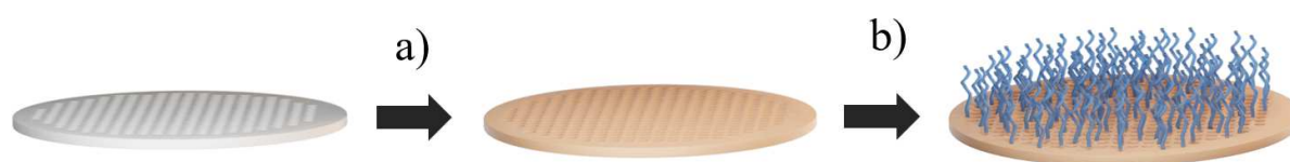
302 Figure 2 – a) Synthesis and coating of polydopamine onto polyethersulfone membrane followed by b) grafting of 303 pH-sensitive PMAA chains through Michael thiol-ene reaction.
