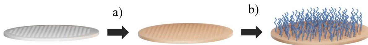
304 Figure 2 – a) Synthesis and coating of polydopamine onto polyethersulfone membrane followed by b) grafting of 305 pH-sensitive PMAA chains through Michael thiol-ene reaction. 306
