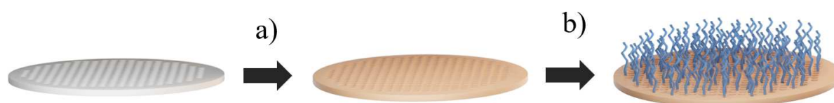
302 Figure 2 – a) Synthesis and coating of polydopamine onto polyethersulfone membrane followed by b) grafting of 303 pH-sensitive PMAA chains through Michael thiol-ene reaction.
