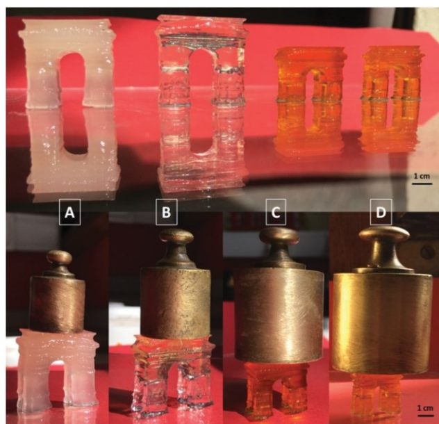
Fig. 4 Swelling in water of triumphal arch samples based on (A) MA 40 POX 66 -PEI 4 , (B) MA 2 POX 120 , (C) MA 2 POX 75 , and (D) MA 2 POX 10 samples (top pictures); Samples bearing the maximum weight before distortion (A) 20 g, (B) 50 g, (C) 100 g, (D) 200 g (bottom pictures).
