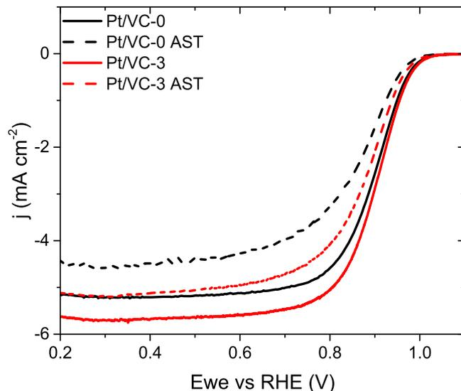
**Figure 11.** Voltammograms in O<sub>2</sub> saturated 1 M HClO<sub>4</sub> at a sweep rate of 20 mV s<sup>-1</sup> at 1600 rpm for Pt/VC-0 and Pt/VC-3 before (full line) and after AST (dashed line).
