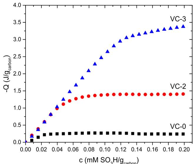
**Figure 6.** Cumulative heat release during titration of Nafion® with non-modified and nitrogen-doped carbon black Vulcan XC72R suspended in water/1-propanol normalised by carbon mass: VC-0 (black squares), VC-2 (red dots) and VC-3 (blue triangles).
