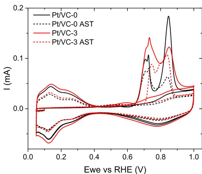
**Figure 10.** Cyclic voltammograms in CO free 0.1 M HClO<sub>4</sub> at a sweep rate of 20 mV s<sup>-1</sup> after CO adsorption for Pt/VC-0 and Pt/VC-3 before (solid line) and after AST (dashed line).
