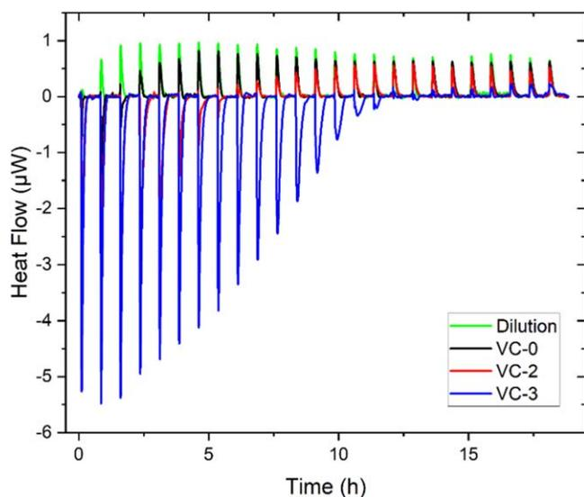
**Figure 5.** Heat flow during titration of Nafion® with non-modified (VC-0) and nitrogen-doped (VC-2, VC-3) carbon black Vulcan XC72R suspended in water/1-propanol or with the solvent mixture as a reference (dilution).
