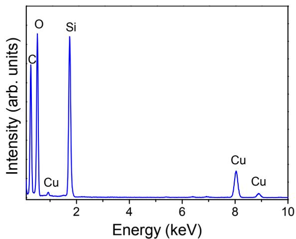
**Fig. 4.** STEM-EDX spectrum in the circular light-colored zone of the PPhA/SiO<sub>2</sub> nanocomposite. The copper peaks are due to the TEM sample grid.
