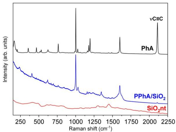
**Fig. 7.** Raman spectrum of PhA, silica nanotubes ( $\text{SiO}_2\text{nt}$ ) and the PPhA/ $\text{SiO}_2$  nanocomposite. The grating used limited acquisition to below  $2300\text{ cm}^{-1}$ .
