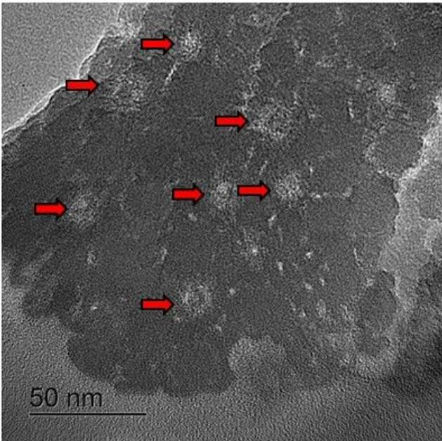
**Fig. 3.** Transmission electron micrographs of the PPhA/SiO<sub>2</sub> nanocomposite. The circular channels at the centers of the nanotubes are indicated by arrows.
