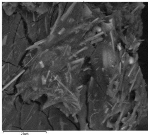
**Fig. 1.** Scanning electron micrograph of the PPhA/SiO<sub>2</sub> nanocomposite.
