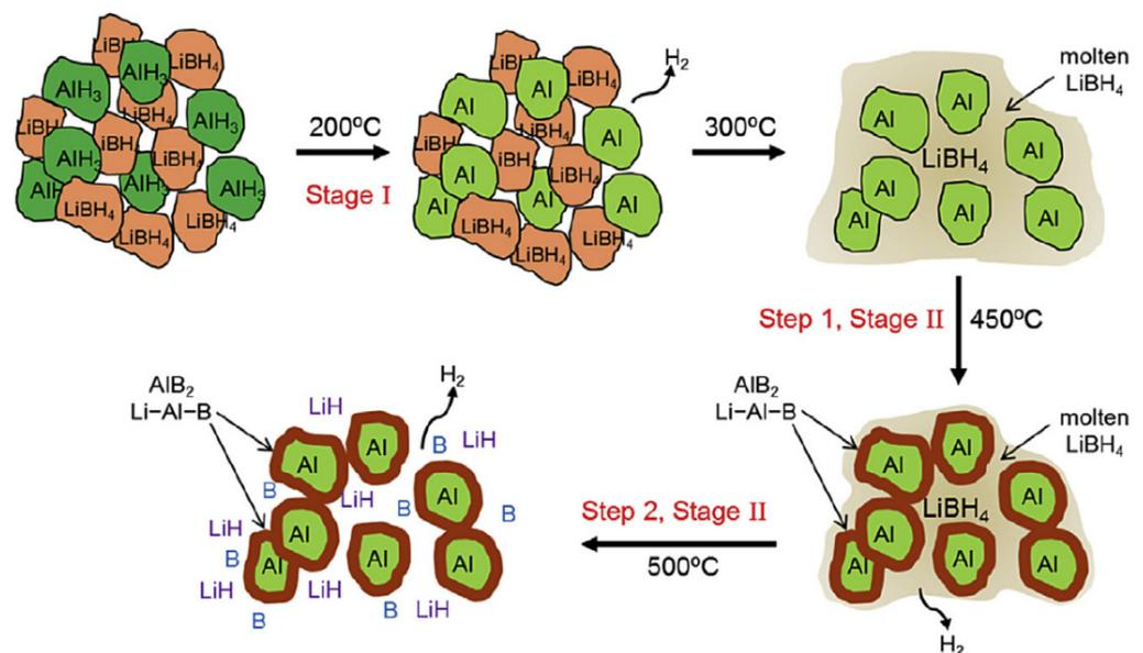
**Figure 7.** Microstructure evolution of a LiBH<sub>4</sub>/AlH<sub>3</sub> composite up to 500 °C, with a heating rate of 4 °C min<sup>-1</sup>. Reprinted with permission from [94]. Copyright (2016), Elsevier.
