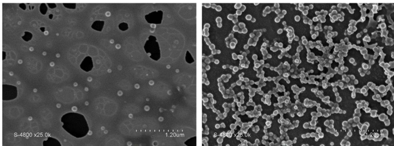
**Figure 18.** Scanning electron microscopy (SEM) micrographs of nanosized AB, dropped onto a carbon film on a cooper grid. Reprinted with permission from [306]. Copyright (2019), American Chemical Society.
