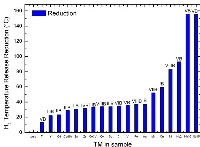
**Figure 11.** Temperature difference between the main decomposition peak of the samples with additives and the one of pure NaBH<sub>4</sub>, observed by TPD. Reproduced with permission from [171].
