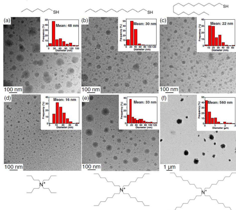
**Figure 10.** TEM images of  $\text{LiBH}_4$  nanoparticles prepared with (a–c) thiol-based surfactants; (d–f) ammonium-based surfactants with different chain lengths. Reprinted with permission from [161]. Copyright (2019), John Wiley and Sons.
