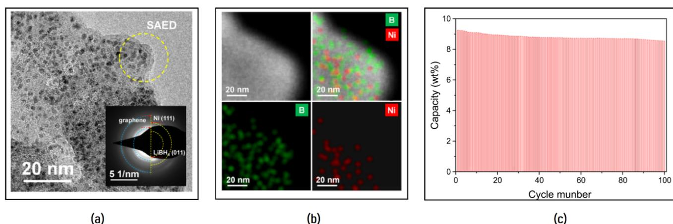
**Figure 8.** (a) Transmission electron microscopy (TEM) image; (b) energy-dispersive X-ray spectroscopy (EDX) mapping and (c) hydrogen cycling stability of nano-LiBH<sub>4</sub> supported on graphene decorated with Ni. Reprinted with permission from [99]. Copyright (2021), Elsevier.
