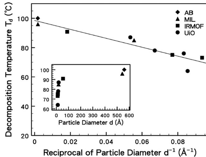
**Figure 16.** Peaked temperatures ( $T_d$ ) of the decomposition of neat AB ( $\diamond$ ), and AB confined in MOF of MIL, IRMOF and UiO MOF vs. the reciprocal particle size ( $d$ ) of the corresponding hydrides.  $T_d$  vs.  $d$  is shown in the inset. Reprinted with permission from [287]. Copyright (2017), American Chemical Society.
