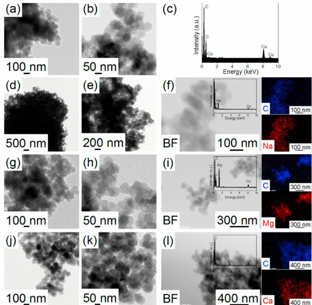
**Figure 13.** Typical TEM images, elemental mapping and EDS analysis of (a–c)  $\text{LiBH}_4$ -HCNs, (d–f)  $\text{NaBH}_4$ -HCNs, (g–i)  $\text{Mg}(\text{BH}_4)_2$ -HCNs and (j–l)  $\text{Ca}(\text{BH}_4)_2$ -HCNs via the melt infiltration method. Reprinted with permission from [136]. Copyright (2019), Elsevier.
