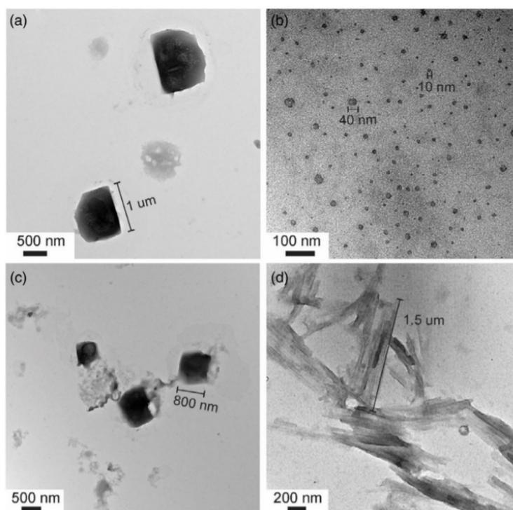
**Figure 12.** Representative TEM images of the  $\text{NaBH}_4$  nanostructures of (a)  $\text{NaBH}_4$ —isopropylamine, (b)  $\text{NaBH}_4$ —tetrabutylammonium bromide, (c)  $\text{NaBH}_4$ —octadecylamine and (d)  $\text{NaBH}_4$ —tridecanoic acid. Reproduced with permission from [191].
