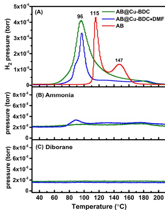
**Figure 17.** Temperature-programmed desorption with mass spectroscopy (TPD-MS) of (A) hydrogen, (B) ammonia and (C) diborane generated from AB (red), AB@Cu-BDC (green) and AB@Cu-BDC-DMF (blue) in the unit of Torr. Reprinted with permission from [288]. Copyright (2019), American Chemical Society.
