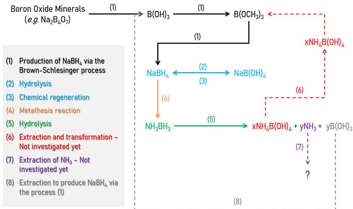
Figure 3. Sodium borohydride vs. ammonia borane for H<sub>2</sub> generation via hydrolysis at ambient conditions.
