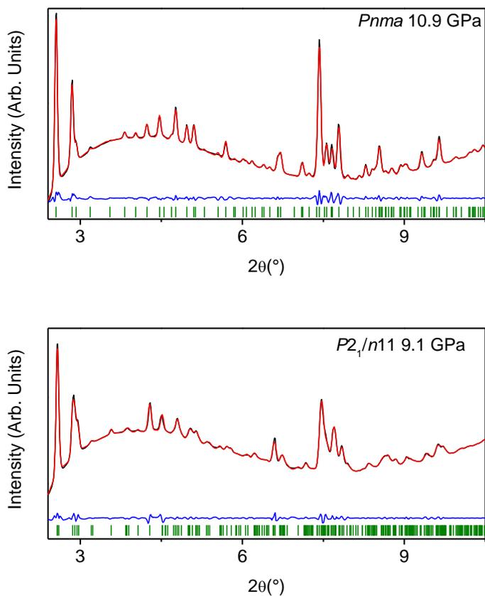
**Figure 3.** Experimental (black), calculated (red) and difference (blue) profiles ( $\lambda=0.4828 \text{ \AA}$ ) for the Le Bail fits for the  $P2_1/n$  structure of MFI/He at 9.1 GPa (below) and for the  $Pnma$  structure of MFI/He at 10.9 GPa (above). Vertical bars indicate the calculated positions of the Bragg reflections.
