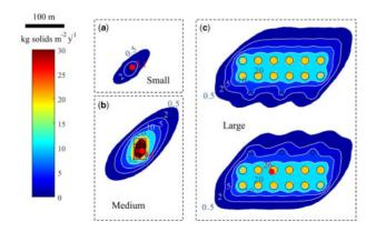
**Figure 8.** Deposition footprint at site 1 for a (a) Small farm, (b) Medium farm, and (c) Large farm. Black squares and circles represent cages. Red circles indicate the maximum deposition rate ( $F_{max}$ ).
