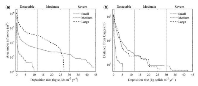
**Figure 9.** Maximum deposition footprints predicted for a variety of hydrodynamic regimes for Small (n = 12 regimes), Medium (n = 15), and Large (n = 27) farms as a function of deposition rate: (a) the largest area under influence and (b) the farthest distance from the cages that any particle was deposited. Vertical dotted lines indicate deposition thresholds for detectable, moderate, and severe impact.
