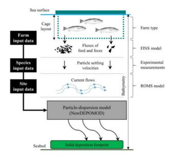
**Figure 2.** Description of the models used and their input data. Dispersion of fish farming waste was predicted with the NewDEPOMOD model using feed and faeces fluxes predicted by the FINS model (Chary *et al.*, 2019), particle-settling velocity data and current flows in Mayotte's North-East Lagoon simulated with ROMS (Chevalier *et al.*, 2017).
