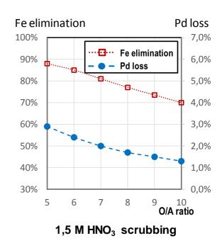
Figure 4: Detailed results of the scrubbing sequence optimization. Initial organic phase: 0,6 M BDMA in toluene, containing Pd (95 mg/L) and Fe (79 mg/L), scrubbed with different aqueous solutions (H<sub>2</sub>O or 1 M HNO<sub>3</sub>) at different organic to aqueous phase volume ratios (O/A). Two scrubbing stages were performed, at same O/A ratio but with possibly different solutions.
