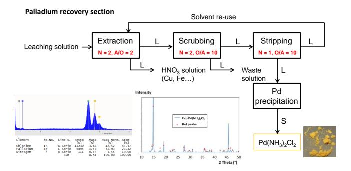
Figure 6: Detailed results of the solvent-extraction processing section of the palladium recovery process (data for other metals not shown for clarity).
