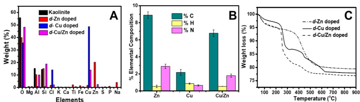
**Fig. 6:** (A) Energy Dispersive X-ray spectra of prepared kaolinite clay and prepared delaminated composites (B) Elemental Analysis of delaminated composites (C) Thermal Gravimetric Analysis of delaminated composites
