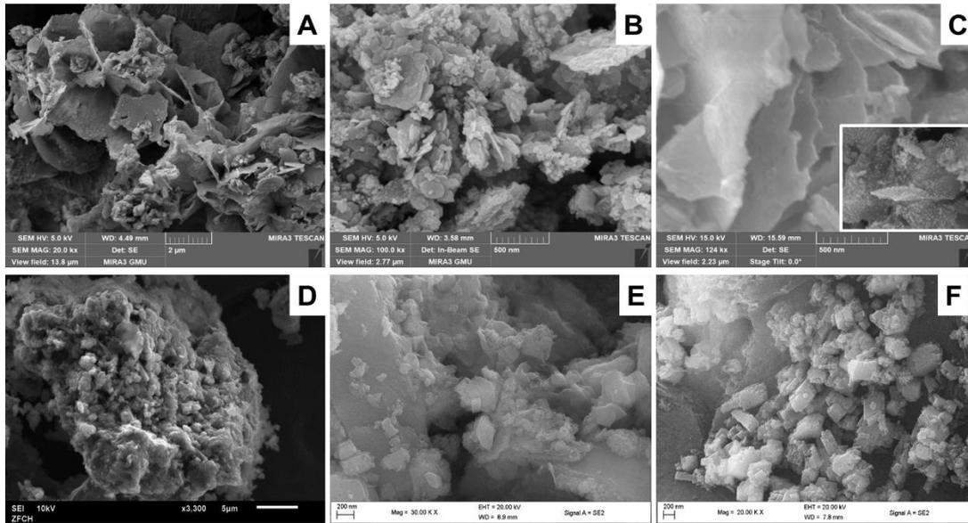
**Fig. 2:** Scanning Electron Microscope Images of (A) *d*-Zn doped (B) *d*-Cu doped and (C) *d*-Cu/Zn doped (D) *f*-Zn doped (E) *f*-Cu doped (F) *f*-Cu/Zn doped Photocatalytic Composites (Figs. 2D-F were reproduced from [22])
