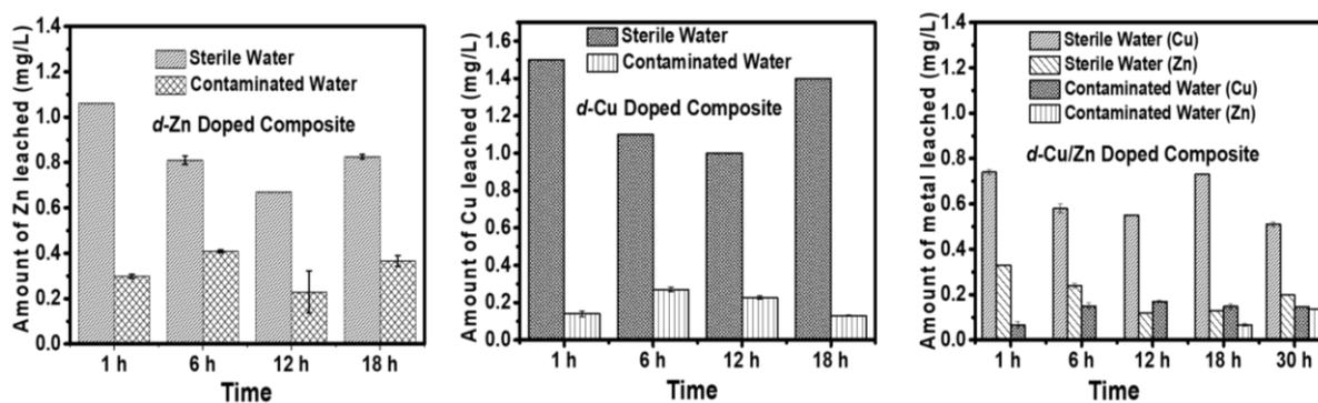
**Fig. 13:** Metal leaching analysis of photocatalytic composite materials at various times during photo-disinfection of water. The error bars represent standard deviation of replicates (n=2)
