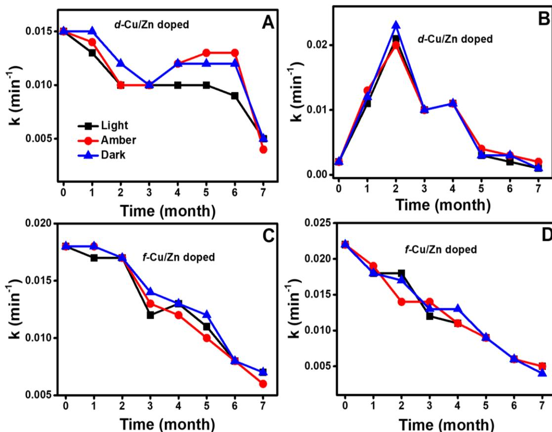
**Fig. 15:** Effect of storage conditions on the rate of photodegradation of Rhodamine B dye using Zn/Cu-doped furnace ( $\text{N}_2$ ) photocatalyst under (A) illumination from fluorescent bulbs and (B) in the dark for 7 months [weight of catalyst = 250 mg; volume = 50 mL, initial conc. of RhB dye = 10 mg/L; time = 120 min].
