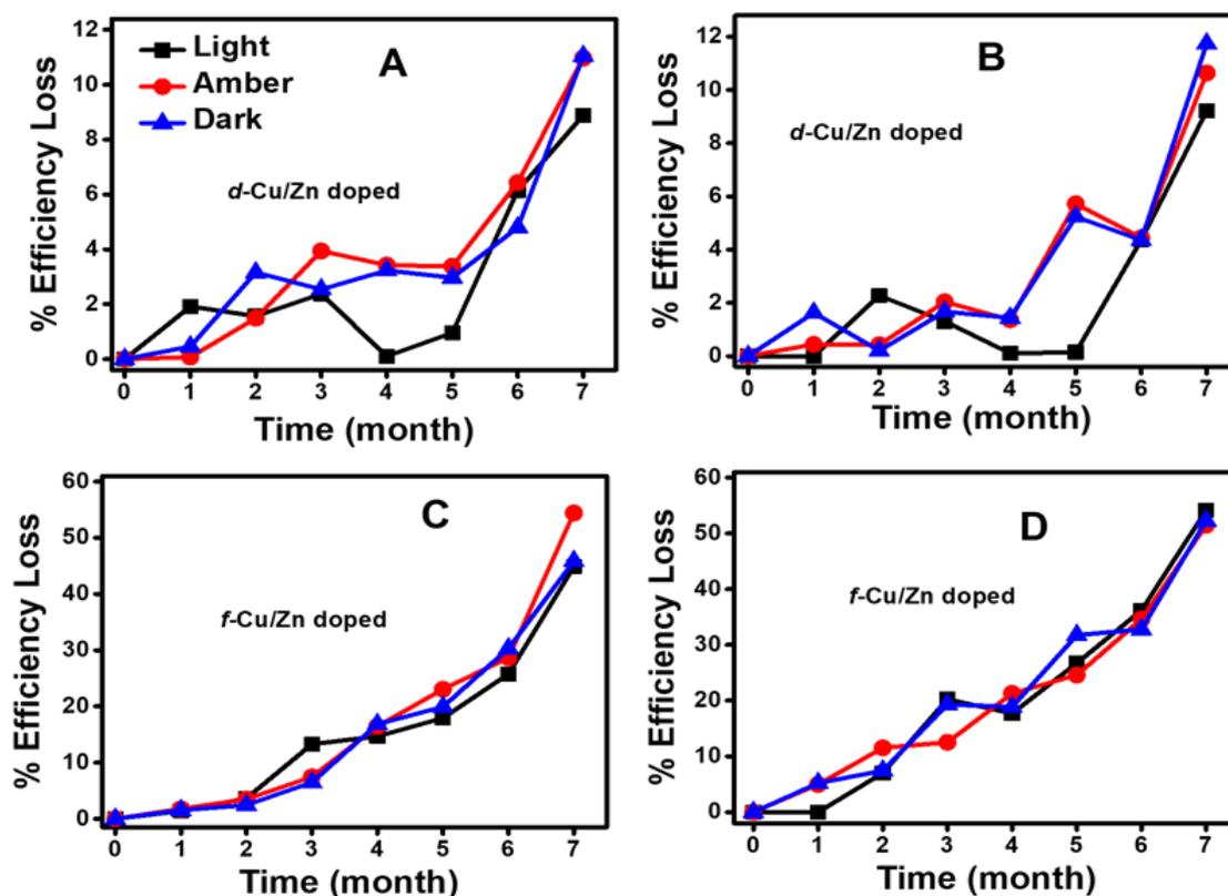
**Fig. 14:** Percentage efficiency loss for *d*-Zn/Cu doped photocatalytic composite (A) under fluorescence illumination (B) in the dark; *f*-Zn/Cu doped photocatalytic composite (C) under fluorescence illumination and (D) in the dark [weight of catalyst = 250 mg; volume = 50 mL, initial conc. of RhB dye = 10 mg/L; time = 120 min].
