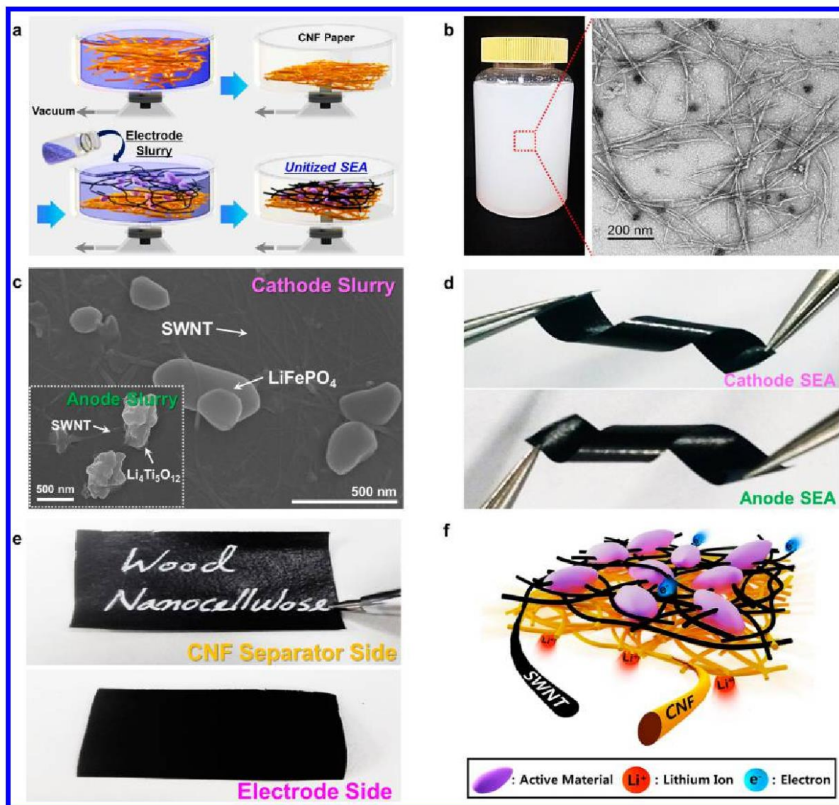
Figure 14. Fabrication of integrated electrode materials as an assembly of CNF (separator material) and single-wall carbon nanotubes (SWNT electrode material). (a) Schematic fabrication procedure for the unitized electrode assembly (b) CNF suspension (left) and a TEM image (right) showing CNFs with nanoscale diameter/length up to a few micrometers. (c) SEM images demonstrating the dispersion state of SWNT and \text{LiFePO}_4 (or \text{Li}_4\text{Ti}_5\text{O}_{12} ) powders in the electrode slurries. (d) Self-standing film of flexible \text{LiFePO}_4 (cathode), and \text{Li}_4\text{Ti}_5\text{O}_{12} (anode). (e) Two faces of CNF separator (top) and \text{LiFePO}_4 cathode (bottom). (f) Conceptual illustration for a 1D nanobuilding block (CNF/SWNT)-enabled structural uniqueness of SEAs, 221 ©American Chemical Society (2014).
