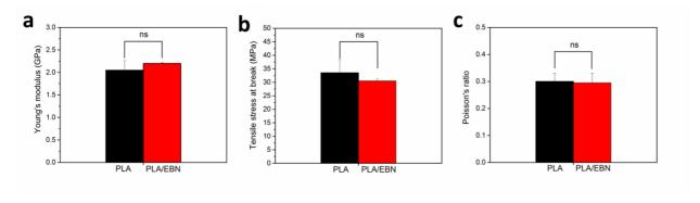
**Figure 4.** Mechanical properties of the scaffolds: (a) Young's modulus, (b) Tensile stress at break, and (c) Poisson's ratio of PLA and PLA/EBN nanocomposites (ns= not significant).
