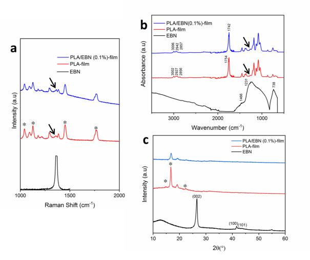
**Figure 2.** Chemical and structural properties of the nanocomposites: (a) Raman spectroscopy, (b) FTIR spectra, and (c) XRD diffractograms of exfoliated boron nitride (EBN), PLA-film, and PLA/EBN nanocomposites.
