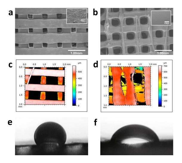
**Figure 5.** Scanning electron micrographs of FDM-based 3D printed PLA and PLA/EBN scaffolds: Top view of the architecture of 3D printed (a) PLA and (b) PLA/EBN scaffolds; inset, zoom showing the surface. Topography of the scaffolds: Representative 3D images of the surface roughness of PLA (c) and PLA/EBN (d) scaffolds. Images showing the contact angle of water on: (e) PLA and (f) PLA/EBN scaffolds.
