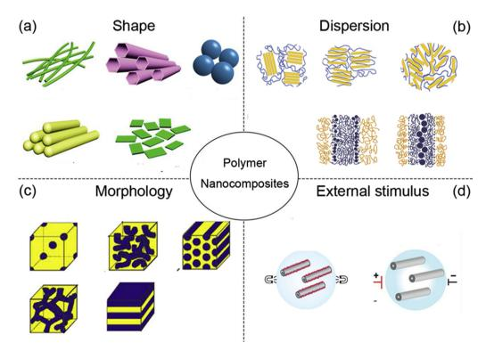
Fig. 3. Research on polymer nanocomposites has focused on (a) shape, (b) dispersion, (c) morphology, and (d) external stimulus. Reproduced with permission from Ref. [29].
