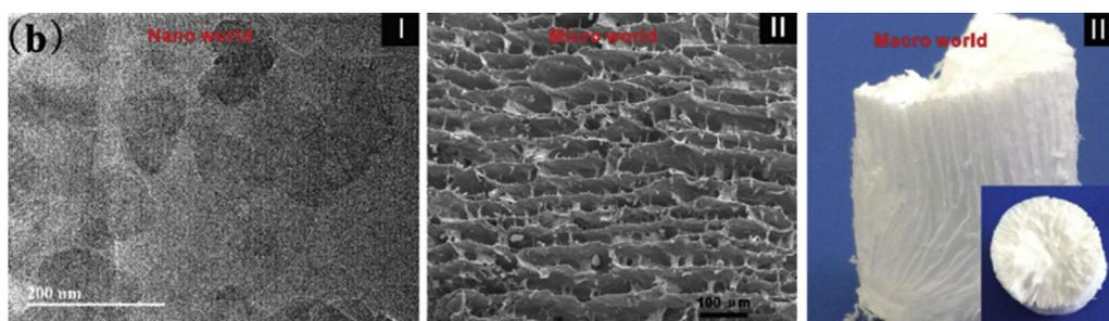
**Fig. 6.** Hierarchical structures of the free-standing 3D-BNNS aerogel: (I) transmission electron microscopy image of the BNNS; (II) scanning electron microscopy image of the 3D-BNNS aerogel in the direction perpendicular to the ice growth; (III) photograph of a 3D-BNNS aerogel. Reprinted with permission from Ref. [41]. Copyright © 2016, WILEY-VCH Verlag GmbH & Co. KGaA, Weinheim.
