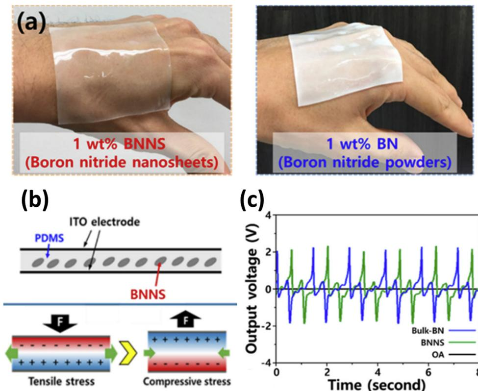
**Fig. 16.** (a) Comparison of the transparency of BNNs and bulk BN in PDMS-based composite devices attached to a human hand. (b) Schematic illustration of the working mechanism of the as-designed TFPS. (c) Open-circuit output voltage signals of BNNs, bulk-BN, and OA samples in PDMS-based composite devices under mechanical vibration (1.5 Hz). OA, oleylamine. Reprinted with permission from Ref. [155]. Copyright © 2018, Elsevier Ltd.
