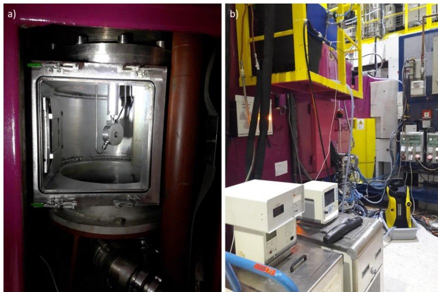
Figure 10: a) Picture of the HP cell mounted on the time-of-flight spectrometer, IN6, at the Institut Laue-Langevin (ILL) b) Picture of the Karcher connected to the HP cell. The flowing water is cooled by two thermostatically-controlled water baths
