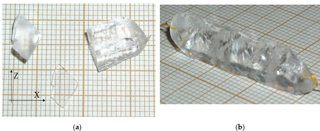
Figure 6. \text{GaPO}_4 crystals grown on x\{12\bar{1}0\} seeds, (a) plate cut perpendicular to Y axis, (b) typical habit of the crystals represented by appearance of the trigonal rhombohedral faces interrupting formation of negative and positive trigonal prism faces.
