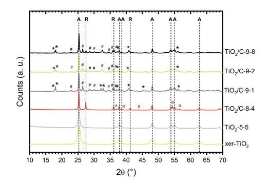
**Figure 4.** X-ray diffraction (XRD) patterns of xer-TiO<sub>2</sub>, TiO<sub>2</sub>-5-5, and the TiO<sub>2</sub>/C-*x*-*y* series. A: Anatase; R: Rutile; \*: Ti<sub>3</sub>O<sub>5</sub> (monoclinic); #: Ti<sub>6</sub>O<sub>11</sub>.
