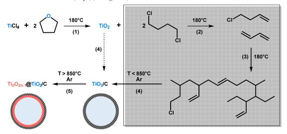
**Figure 1.** Schematic representation of the non-hydrolytic sol-gel (NHSG) route developed herein to prepare TiO<sub>2</sub>, TiO<sub>2</sub>/C and Ti<sub>n</sub>O<sub>2n-1</sub>@TiO<sub>2</sub>/C nanocomposites. (1) Alkoxylation/Condensation; (2) Dehydrochlorination; (3) Polymerization; (4) Carbonization; and (5) Partial carbothermal reduction. In this representation, xer-TiO<sub>2</sub> corresponds to TiO<sub>2</sub> together with organic by-products (box on the right side) before step (4).
