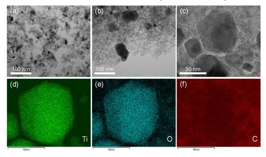
**Figure 6.** Transmission electron microscopy (TEM) images of (**a**) xer-TiO<sub>2</sub> and (**b**) TiO<sub>2</sub>/C-9-1. (**c**) High resolution TEM image and (**d**–**f**) STEM-EDX mapping of TiO<sub>2</sub>/C-9-1. The corresponding element (Ti, O or C) is noted in the bottom left corner of each image.
