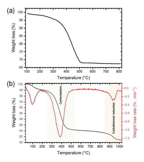
**Figure 2.** Thermogravimetric analyses performed (**a**) under synthetic dry air flow (50 mL min<sup>-1</sup>) and (**b**) under argon flow (50 mL min<sup>-1</sup>) at 10°C min<sup>-1</sup> of xer-TiO<sub>2</sub>.
