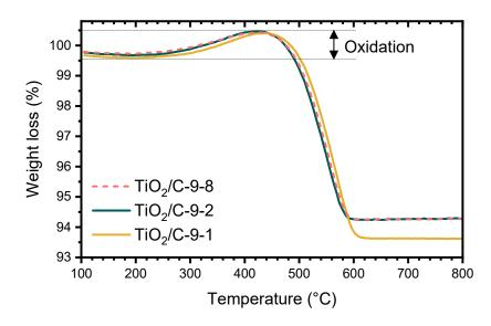
**Figure 3.** Thermogravimetric analyses (TGA) performed under synthetic dry air flow (50 mL min<sup>-1</sup>) at 10 °C min<sup>-1</sup> of TiO<sub>2</sub>/C-9-*y* samples.
