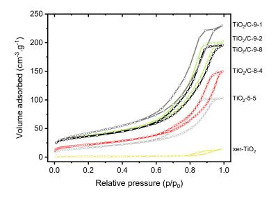
**Figure 5.** Nitrogen sorption isotherms at 77 K of xer-TiO<sub>2</sub>, TiO<sub>2</sub>-5-5 and the different TiO<sub>2</sub>/C-*x*-*y* samples prepared herein.
