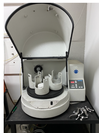
Figure 1. Fritsch-pulverisette 5, a planetary ball mill.
