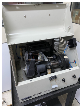
Figure 3. SPEX Mixer/Mill 8000 ball mill.
