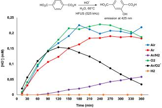
Scheme 3. Titration of •OH radical using TPA (2 mM) as a function of the gaseous atmosphere. \*The decrease in the •OH radical amount with time under Ar/O $_2$  is due to the large production of •OH radicals which degrade TPA-OH used as a probe.
