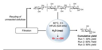
Scheme 1. Depolymerisation of cellulose to glucose induced by HFUS.
