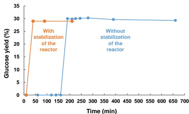
Scheme 2. Kinetic profile of the reaction recorded at 60 °C under air (525 kHz, acoustic power: 0.36  $\text{W}\cdot\text{mL}^{-1}$ ). Cellulose was introduced before (blue) or after (orange) warm-up of the reactor
