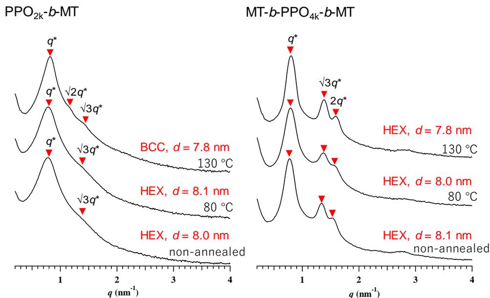
Figure 3. SAXS profiles of the bulk  $\text{PPO}_{2k}\text{-}b\text{-MT}$  and  $\text{MT-}b\text{-PPO}_{4k}\text{-}b\text{-MT}$  samples before and after thermal annealing at 80 and 130 °C for 30 min. All SAXS experiments were performed at room temperature.
