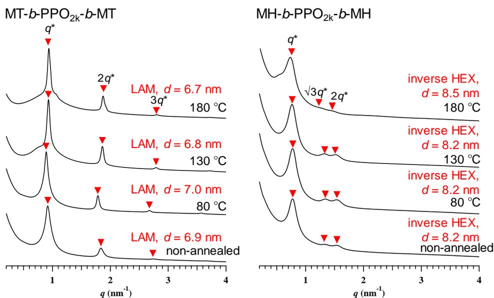
Figure 4. SAXS profiles of the bulk  $\text{MT-}b\text{-PPO}_{2k}\text{-}b\text{-MT}$  and  $\text{MH-}b\text{-PPO}_{2k}\text{-}b\text{-MH}$  samples before and after thermal annealing at 80, 130, and 180 °C for 30 min. All SAXS experiments were performed at room temperature.
