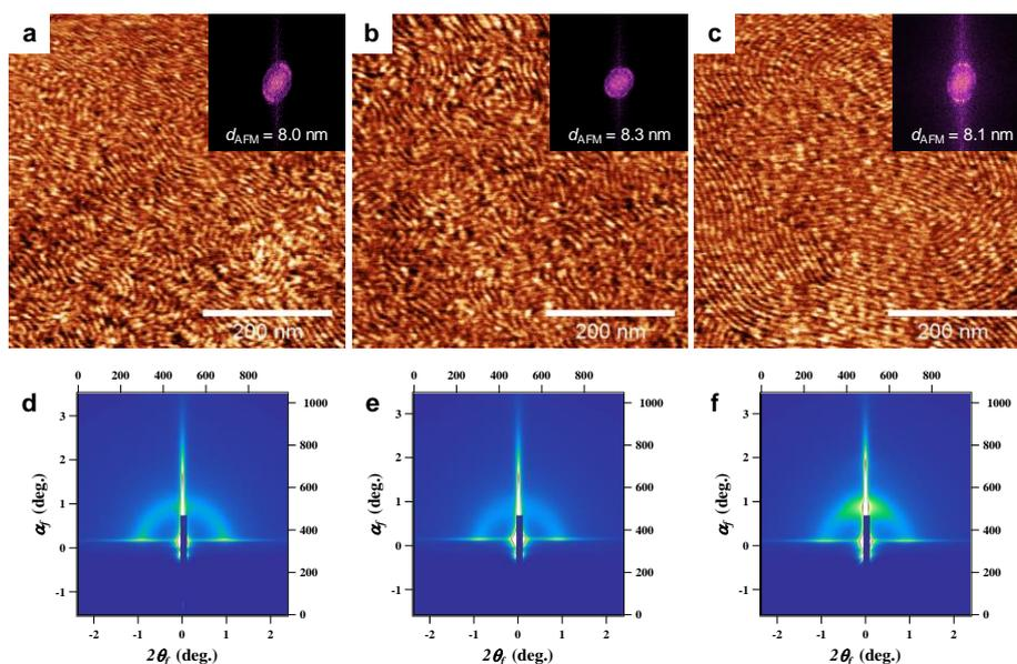
Figure 7. AFM phase images of MT-*b*-PPO<sub>4k</sub>-*b*-MT before and after thermal annealing at different temperatures: (a) as-cast sample and samples annealed at (b) 80 and (c) 130 °C for 30 min; (d), (e), and (f) are their corresponding synchrotron GISAXS profiles. The insets in the AFM images show the corresponding FFT patterns, from which the  $d_{\text{AFM}}$  was estimated. The thin films were prepared by spin coating a 2 wt% copolymer solution in ethanol onto a silicon substrate.
