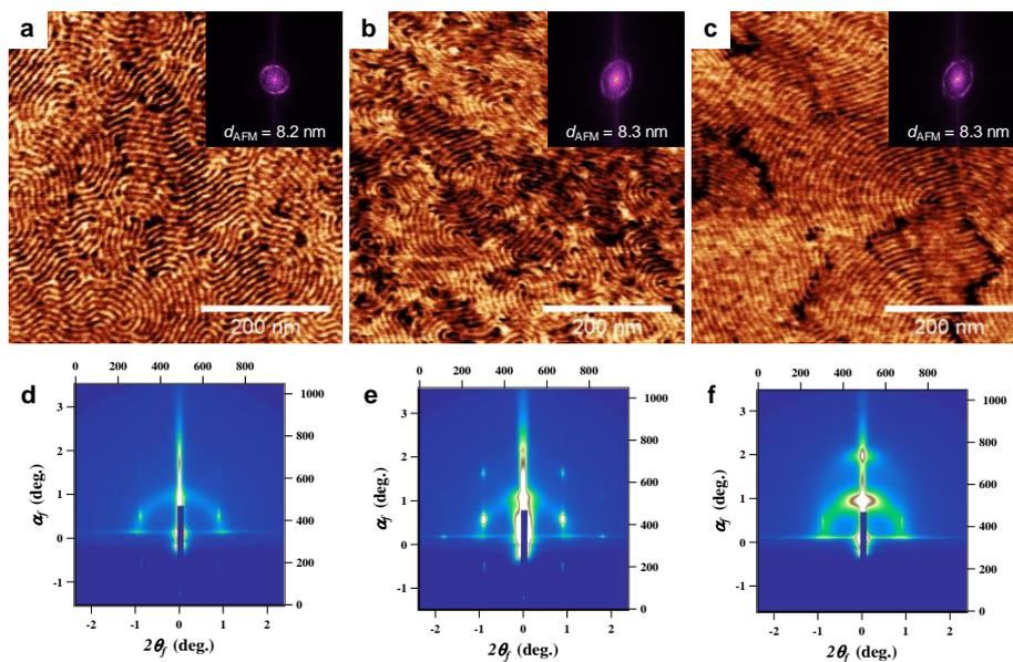
Figure 6. AFM phase images of PPO<sub>2k</sub>-*b*-MT before and after thermal annealing at different temperatures: (a) as-cast sample and samples annealed at (b) 80 and (c) 130 °C for 30 min; (d), (e), and (f) are their corresponding synchrotron GISAXS profiles. The insets in the AFM images show the corresponding FFT patterns, from which the  $d_{AFM}$  was estimated. The thin films were prepared by spin coating a 2 wt% copolymer solution in ethanol onto a silicon substrate.
