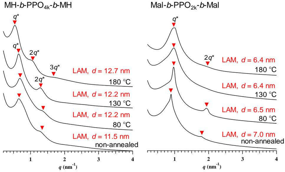
Figure 5. SAXS profiles for the bulk MH-*b*-PPO<sub>4k</sub>-*b*-MH and Mal-*b*-PPO<sub>2k</sub>-*b*-Mal samples before and after thermal annealing at 80, 130, and 180 °C for 30 min. All SAXS experiments were performed at room temperature.
