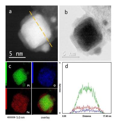
**Figure 2.** STEM-EDXS characterization of a single Pt-rich particle in Pt<sub>2.0</sub>Fe<sub>1.0</sub>d. a) HAADF and b) bright field images, c) EDXS elemental mapping for Pt (green), iron (red), oxygen (blue) and overlay Pt and Fe (lower left hand side corner), d) intensity profiles of the various elements along the line indicated in a).
