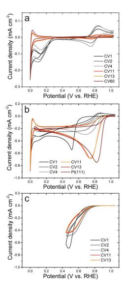
**Figure 3.** Cyclic voltammograms of the 3.2-Fe<sub>2</sub>O<sub>3</sub>/Pt(111) film in (a) Ar-saturated and (b-c) O<sub>2</sub>-saturated 0.1 M HClO<sub>4</sub> solution at a scan rate of 20 mV·s<sup>-1</sup> between (a-b) 1.05 and 0.0 V vs. RHE and (c) 1.05 and 0.45 V vs. RHE.
