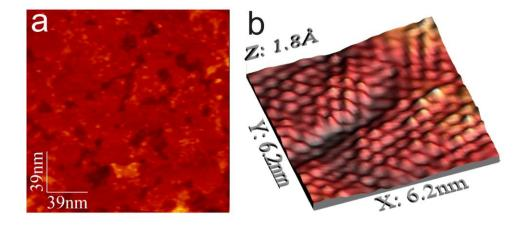
**Figure 4.** Low- (a) and high-resolution EC-STM images (b) of 1.6-Fe<sub>2</sub>O<sub>3</sub>/Pt(111) in Ar-saturated 0.1 M HClO<sub>4</sub> solution at 1.05 V vs. RHE. Tunneling parameters:  $U_b = -900$  mV,  $I_t = 4.8$  nA (a) and  $U_b = -697$  mV,  $I_t = 4.8$  nA (b).
