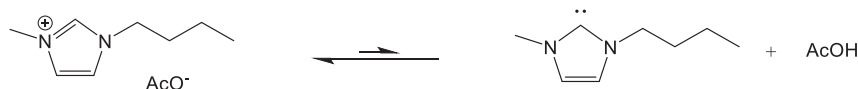
Scheme 1. Deprotonation of butylmethylimidazolium (BMIM) cation with acetate anions and formation of a N-heterocyclic carbene ( right ).
